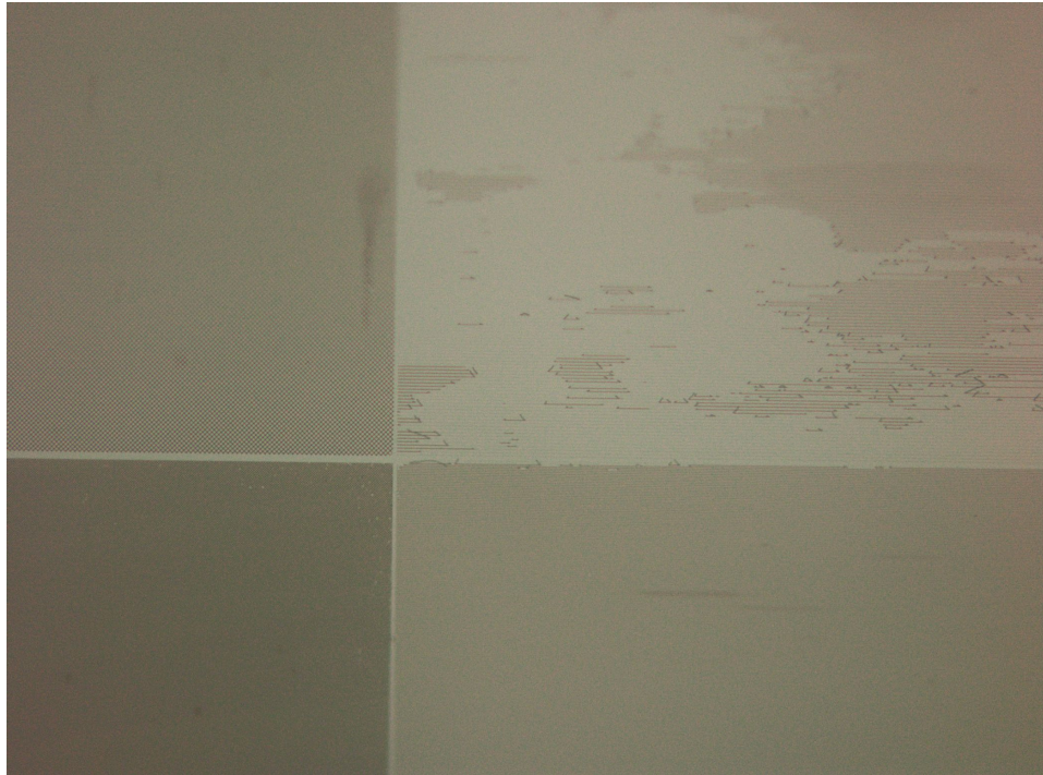
Figure 3.47: Eighth imprint of 200 nm structures with TMPTA at 20x magnification. Some of the features are missing.
