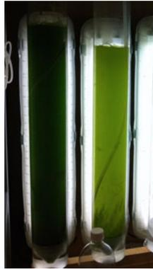
**Figure 3.2.:** *Algae cultivation tubes with a timer controlled illumination. Each tube fits 3 litres of algae culture and the aeration can be adjusted for each tube.*
