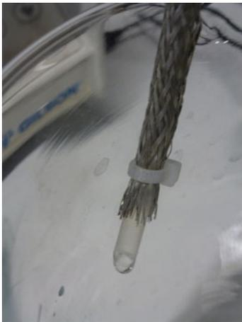
**Figure 5.9:** One end of a PVC tube that connects the peristaltic pump with the detection module; coated with steel to prevent electro-magnetic interferences.
