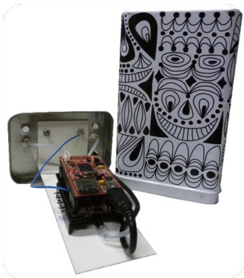
**Figure 5.3.:** Device made out of POM-C installed on a cardboard to store it in the metal box during the measurements. Besides, the device is grounded on the metal box.
