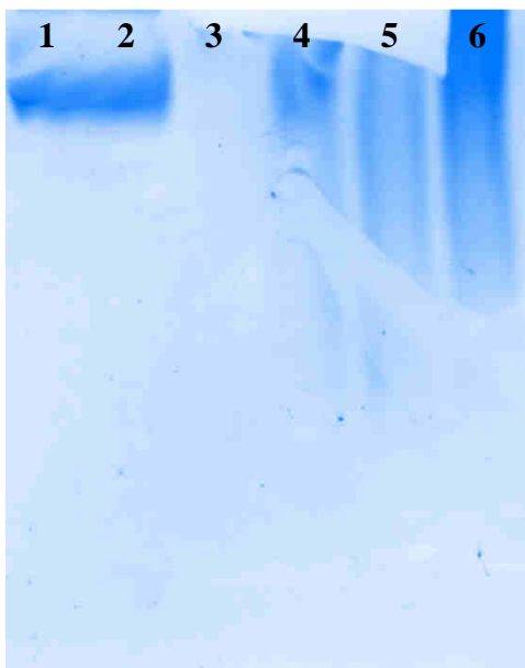
Fig. 3-25: vertical agarose gel electrophoresis 1.4% towards cathode (TKU)
