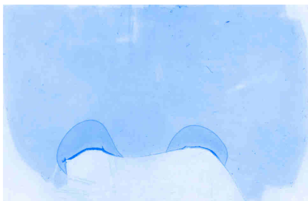
Fig. 3-32: 1.8% agarose towards anode; gel casted without buffer (TKU)
