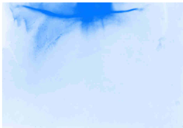
Fig. 3-33: 1.8% agarose towards cathode; gel casted without buffer (TKU)
