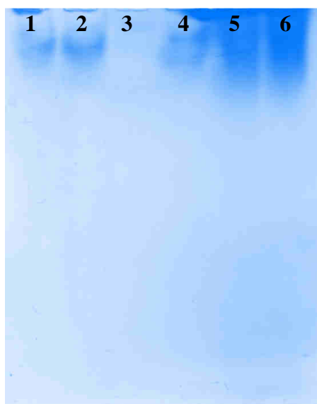
Fig. 3-35: 1.8% agarose towards cathode; gel casted with \frac{1}{2} x running buffer (TKU)
