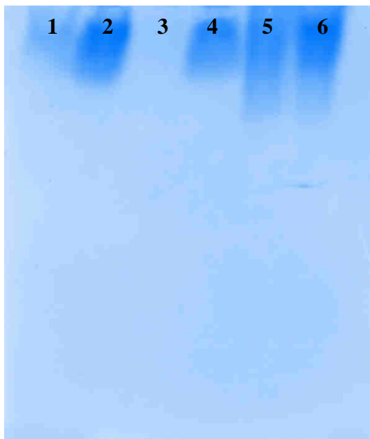
Fig. 3-21: vertical agarose gel electrophoresis 2% towards cathode (TKU)
