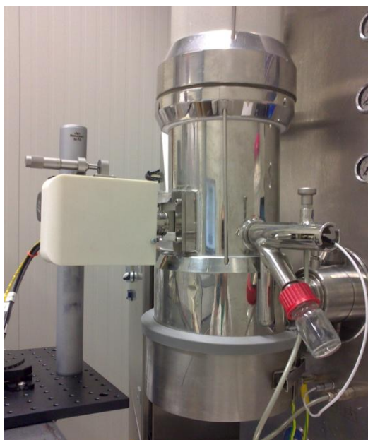
Fig. 5.3. Positioning of the OCT sensor
