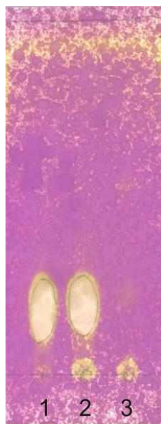
Figure 5.3: Thin layer chromatography to check dialysis performance; lane 1: 5 % (w/v) sorbitol positive control; lane 2: undialyzed rhG-CSF bulk solution containing 5 % (w/v) sorbitol; lane 3: dialyzed rhG-CSF solution
