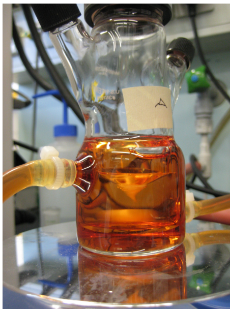
Figure 5.1: A magnetic stir bar in a miniature bioreactor was used for stirring experiments. 15 ml of 1.39 \pm 0.03 mg/ml rhG-CSF solution was stressed for 47 hours at 25°C
