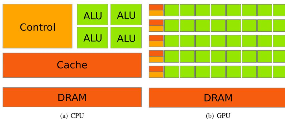
**Figure 6.1:** Architecture of CPUs vs. architecture of GPUs [Nvidia, 2009]. In CPUs, a large portion of the total transistors are dedicated to flow control and memory caching. GPUs put less emphasis on flow control and caching but provide a large amount of ALUs for massively data-parallel computations.
