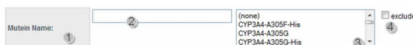
Figure 4.6: Snippet of search parameter selection. (1) Property name. (2) Selection aid input field simplifies browsing within the list box (3). (3) List box containing all available values for the correlated property. Selected value can be inverted by tagging exclude check box(4).
