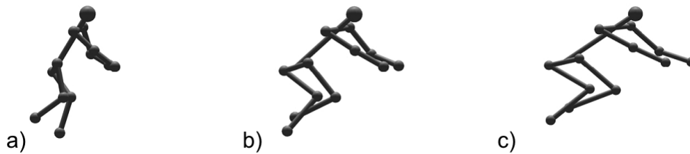
Figure 5.5: Impact of the scale factor s on the estimation. The scale is increasing from left to right. Image from [28]
