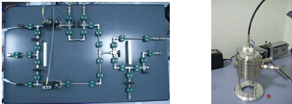
Figure 7.1: Top left: Ready made device; Top right: Measurement cell with gas in and outlet; Bottom left: Gas mixing and humidity measurement setup; Bottom right: Measurement cell with a rack for the fiber optics to the detector.
