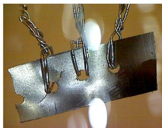
**Figure 4.9:** Sample cracked during the measurement
