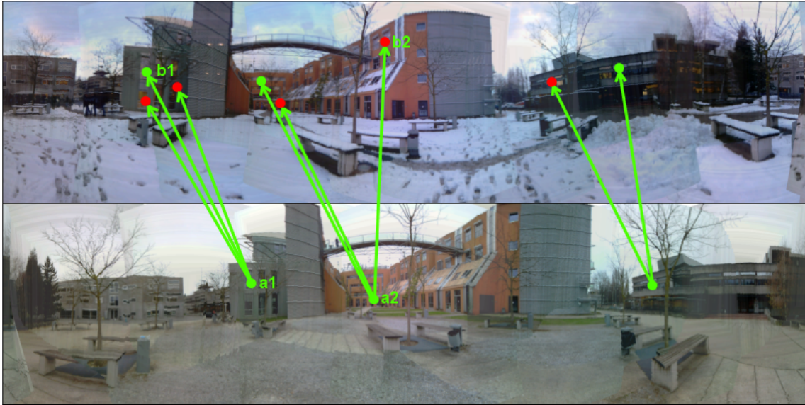
Figure 5.9: We use the four positions a1 , b1 , a2 , b2 as input for the RANSAC algorithm. The points a1 and a2 are the position in the stored database panorama. The point b1 belongs to one of the three best matches of the annotation a1 , the same is true for b2 and a2 . These four points are converted to 3D vectors in the cylindrical map and are used for the rotation calculation as we show in Figure 5.8.
