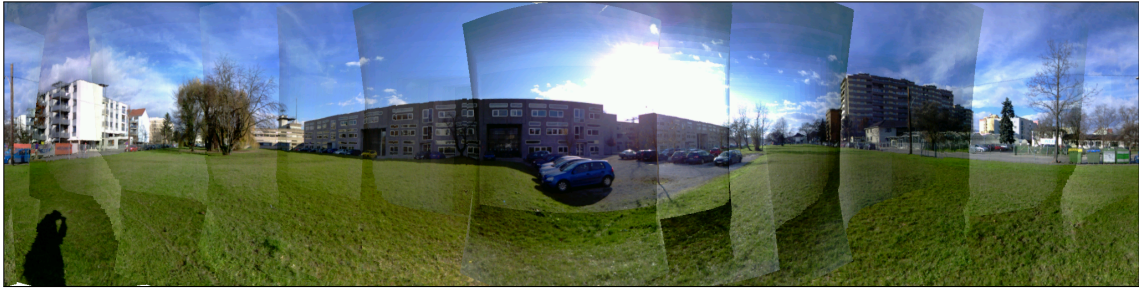
Figure 5.5: This image shows the artifacts which occur because of automatic exposure adjustment of current mobile phone cameras.
