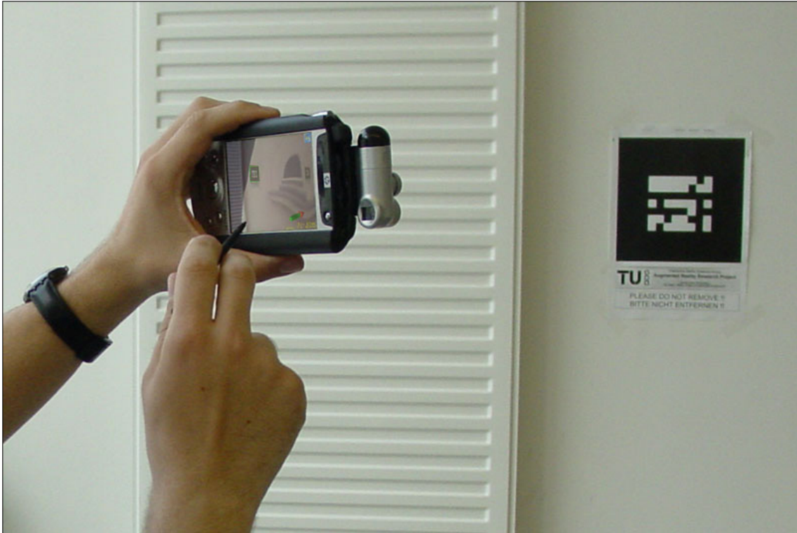
Figure 2.1: Marker-based AR system by Wagner et al. [31] running on a PDA
