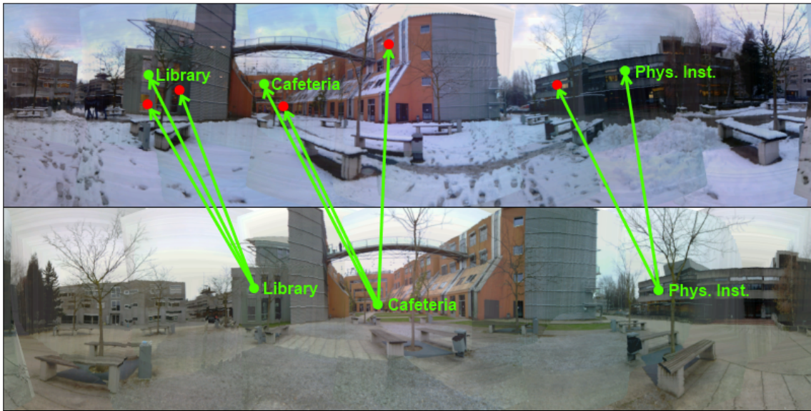
Figure 5.7: This Figure shows a panorama with according annotations stored on our content server (bottom) and a new created panorama where the annotations are tried to be matched (top). For every annotation we store a maximum of three best matches. The green dots in the upper image have the best matchings scores and are therefore used for label placement. The red ones are the second and third best matches of an annotation which makes them suitable for a possible correct match.
