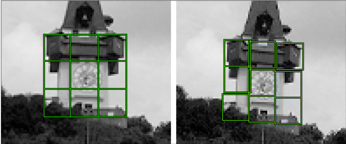
Figure 3.5: Annotation template consisting of 9 image patches in a 3x3 configuration. This makes annotation matching more robust against small position changes. For further details see Langlotz et al. [18]
