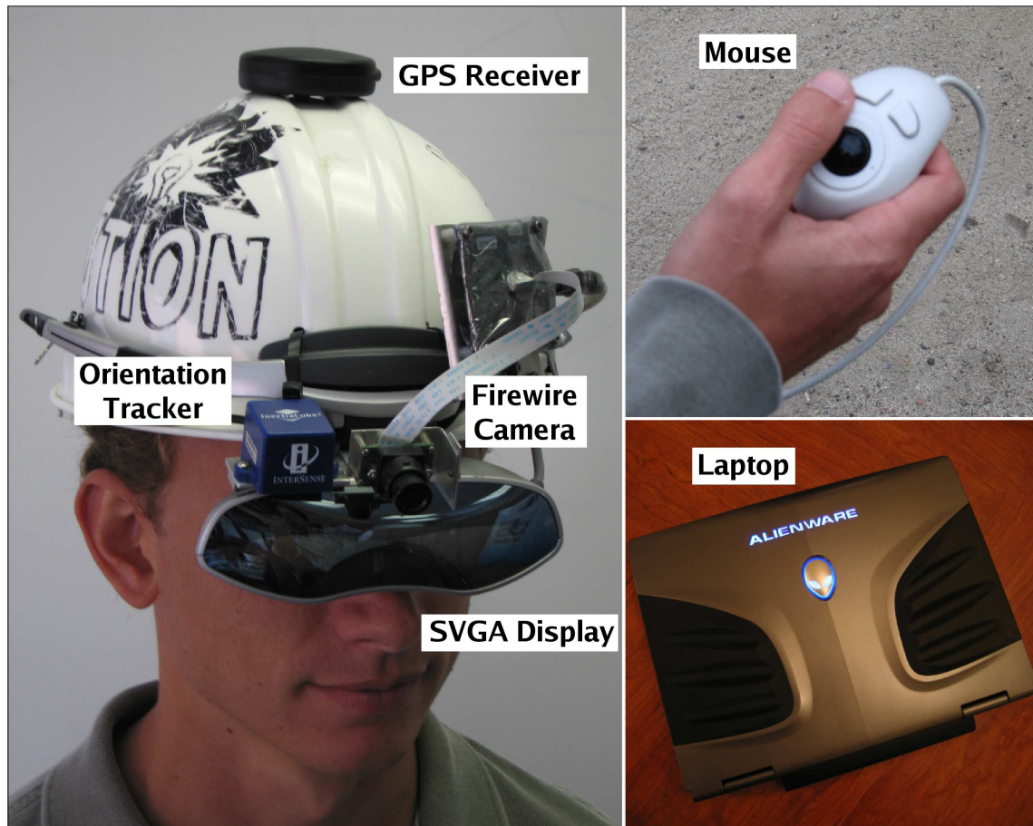
Figure 1.1: This Figure shows an example of a mobile AR system composed out of a backpack computer with Head Mounted Display by Wither et al. [37]
