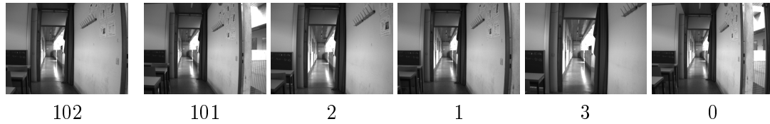
Figure 5.8: Loop Detection. The first image is the query image. The other five images are the nearest neighbors (NN) in ascending order. The numbers below the images denote the corresponding keyframe number. The query image is keyframe 102 and the first NN in image space is the keyframe quite recently stored. All other NN are stored a long time before.
