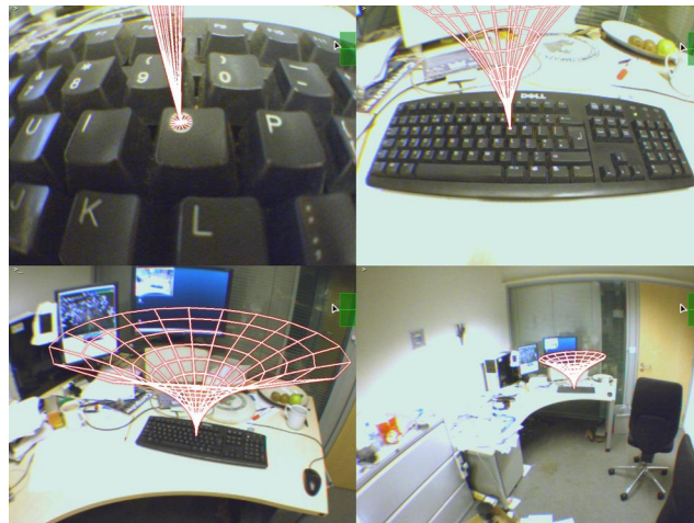
Figure 2.5: Example of a scene tracked by PTAM. PTAM is initialized on the upper right image and is then moved closer and further from the initialized object (taken from [19]).
