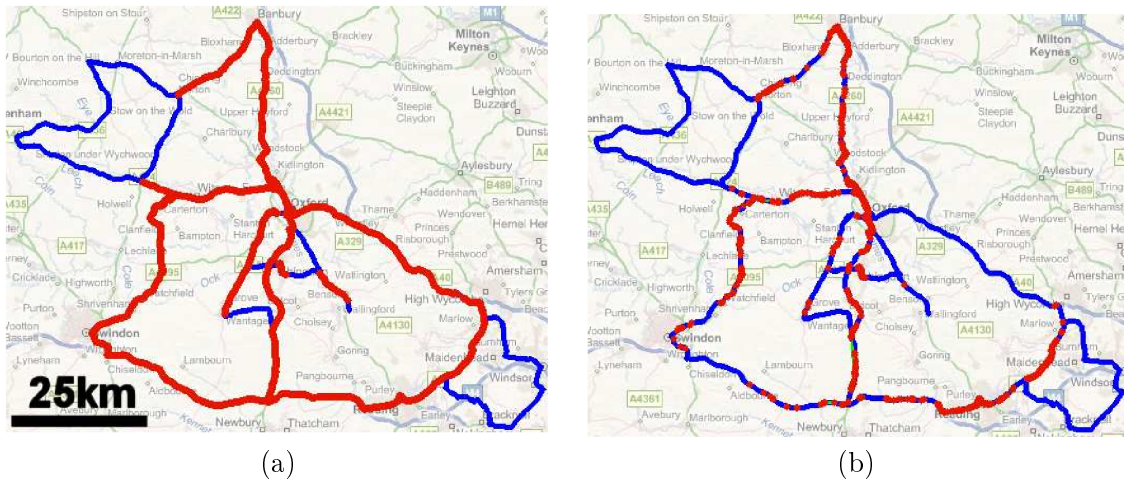
Figure 2.4: FAB-MAP Experiment. (a) The groundtruth of a large trajectory. Blue parts of the trajectory are visited only once, whereas the red parts are visited at least two times. (b) The detected loop closures are shown in blue taken from [7].
