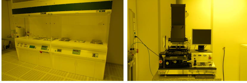
Figure 2.1: Wet bench and EVG 620 mask aligner for photolithography in the clean room at NTC Weiz.
