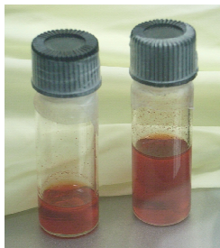
Figure 3.2: Solutions of carbazole-based polymer P7 with 2g/l in THF (left) and 1g/l in \text{CHCl}_3 (right).
