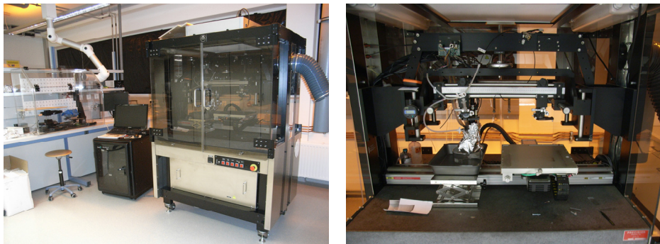
Figure 2.4: ITI XY MDS Printer with Apollo II printhead support kit (left) and interior of the inkjet printer with separated heating units for ink and substrate (right).
