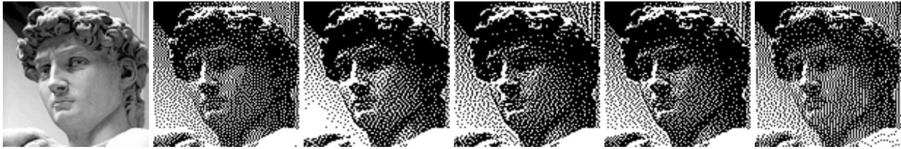
Figure 5.15: These images are generated using different dithering algorithms: Original image, 'Floyd-Steinberg', 'Atkinson', 'Jarvis, Judice and Ninke', 'Stucki' and 'Variable Constants'. (Original image from Dominique Tous-saint)
