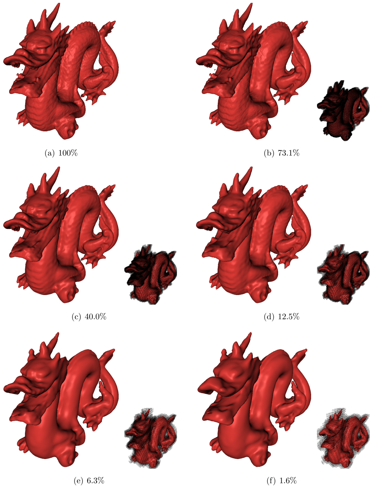
Figure 6.7: Dragon dataset: View dependent Wavelet Reconstruction greatly reduces rendering time (see Table 6.4), while retaining good visual quality.
