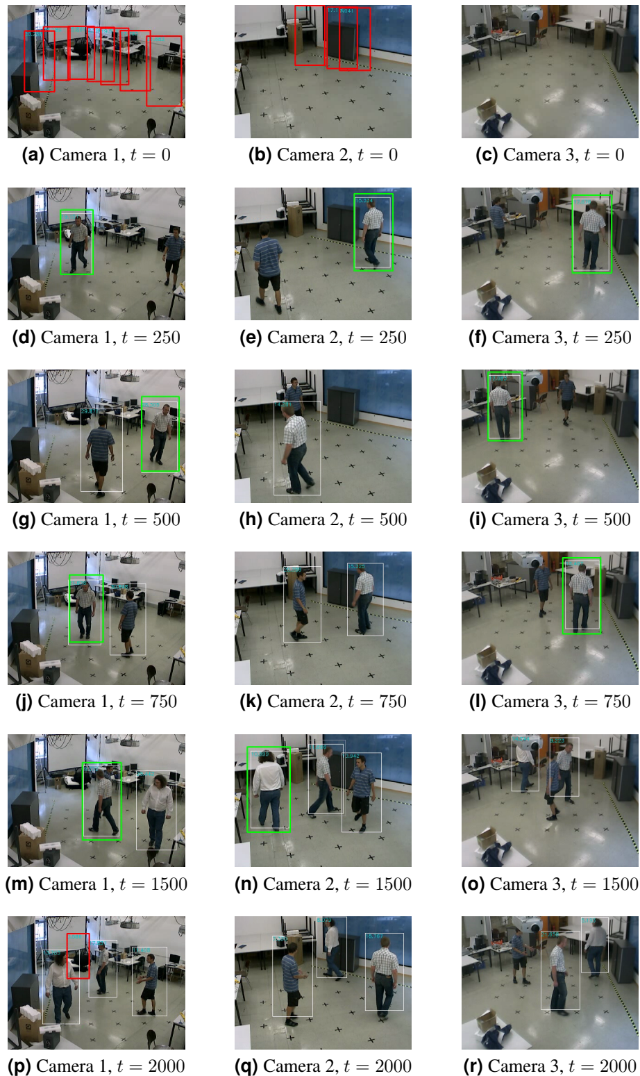
Figure 6.2: Training process using three cameras on the DT2 - Set4 dataset. White bounding boxes are detections in the single camera views. Red bounding boxes correspond to negative updates that are obtained with a background updates that are obtained using the centralized approach and green bounding boxes correspond to positive updates that are obtained using the centralized approach. Grey bounding boxes indicate suppressed updates.
