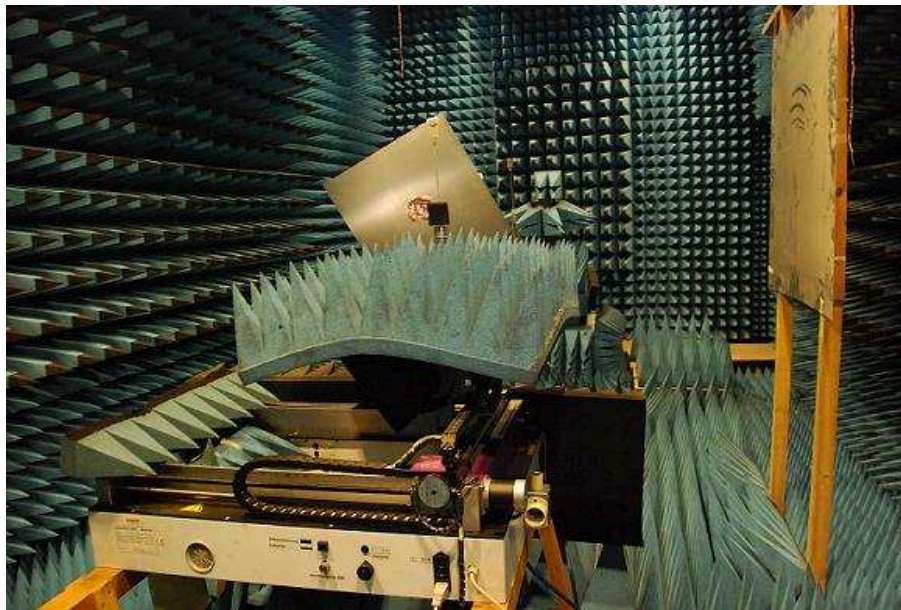
Figure 3.1: Reflection Environment for Scenario 3 with two reflectors and positioning device
