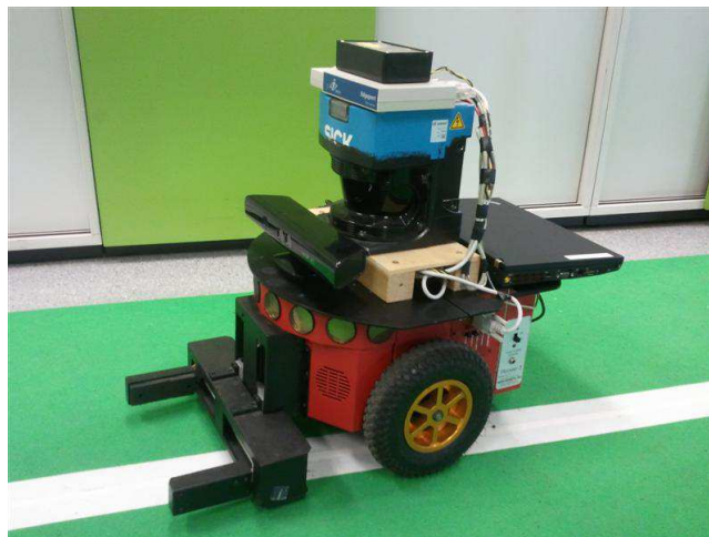
Figure 3.1: Pioneer P3-DX platform with equipment at the Institute for Software Technology, Graz University of Technology
