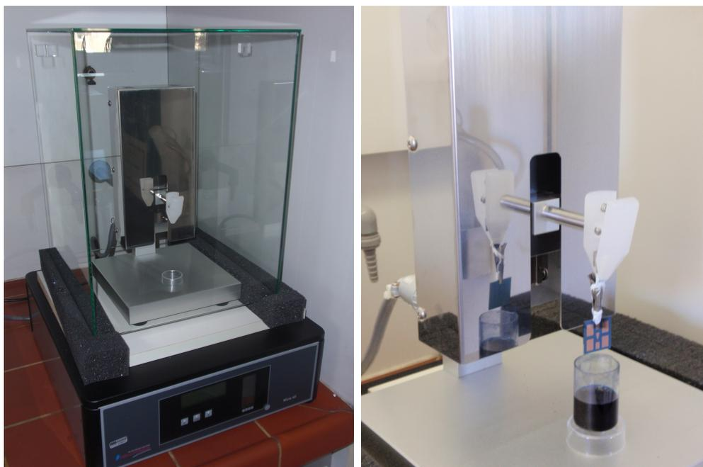
Figure 4.1.: Basic setup of a dip coating instrument. Left: The dip coater is located on an active isolation/vibration table to decrease outside influences. Right: The device is held by a Teflon clip and pulled out of the solution slowly.
