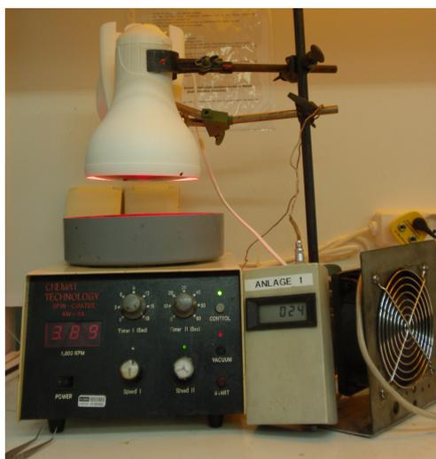
Figure 4.12.: Top: Schematic illustration of the spin coating setup including an IR lamp to heat the substrate. Bottom: Picture of the real setup. The fan on the right hand side is responsible for cooling the spin coater to reduce its temperature.
