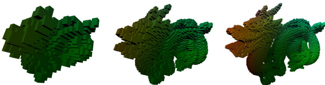
Figure 2.10: Representation of the Stanford dragon model as voxel grid at different grid resolutions. Depending on the resolution the approximation becomes more accurate or less accurate. Coarser approximations allow for a quicker but less accurate lighting computation. The image is originally published in [RBA09].
