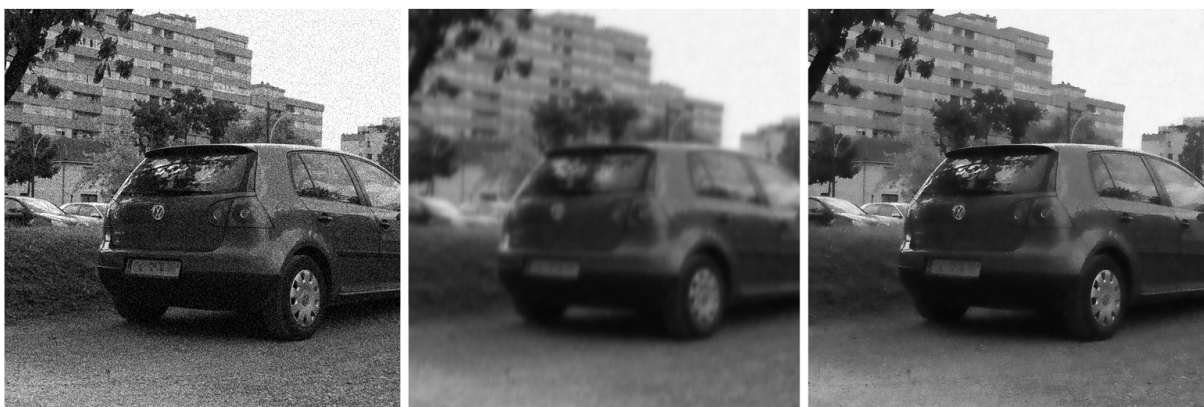
Figure 3.4: First image: Photo of a car with a bit of noise added. Second: The result of blurring the photo with a gaussian filter of size 21 \times 21 and a parameter \sigma_s = 3.0 . The noise is gone but so is most of the detail as well. Third: Result of a bilateral filter of size 21 \times 21 with \sigma_s = 3.0 and \sigma_r = 32.0 . The noise is reduced greatly while the edges of the details like the building or the tree leaves are preserved.
