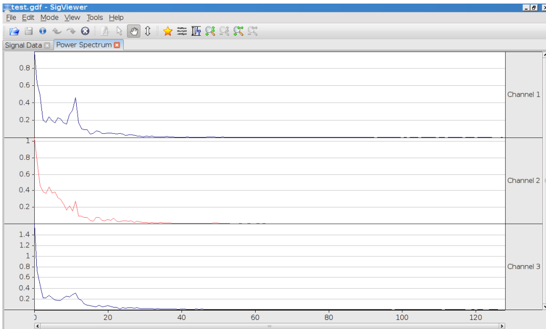
Figure 3.5: Screenshot of SigViewer displaying a Power Spectrum. The unit of the x-axis is Hz. The unit of the y-axis is \frac{\mu V^2}{Hz} .
