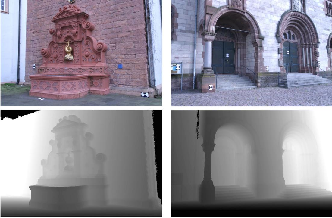
Figure 5.1: **Reference Depth Maps from Lidar Ground Truth:** Reference depth maps generated from the ground truth models acquired by Lidar for one image of the fountain-P11 image sequence (left) and Herz-Jesu-P8 (right) from Strecha et al. [37].
