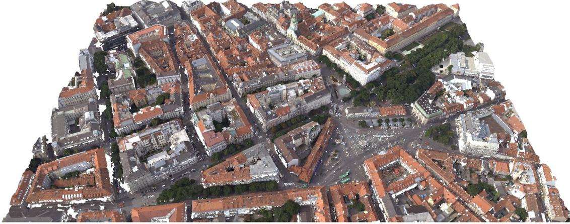
Figure 1.1: **A Reconstructed Scene:** The scene has been reconstructed from five Microsoft VEXCEL UltraCam Images from the Jakomini dataset. The images have a geometrical resolution of 7500x11500 pixels with approximately eight centimeter ground resolution per pixel.
