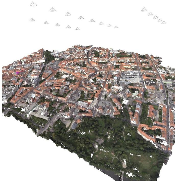
Figure 3.1: **Reconstruction from Aerial Images:** Illustration of a city model from the Jakomini dataset including the reconstructed camera positions.
