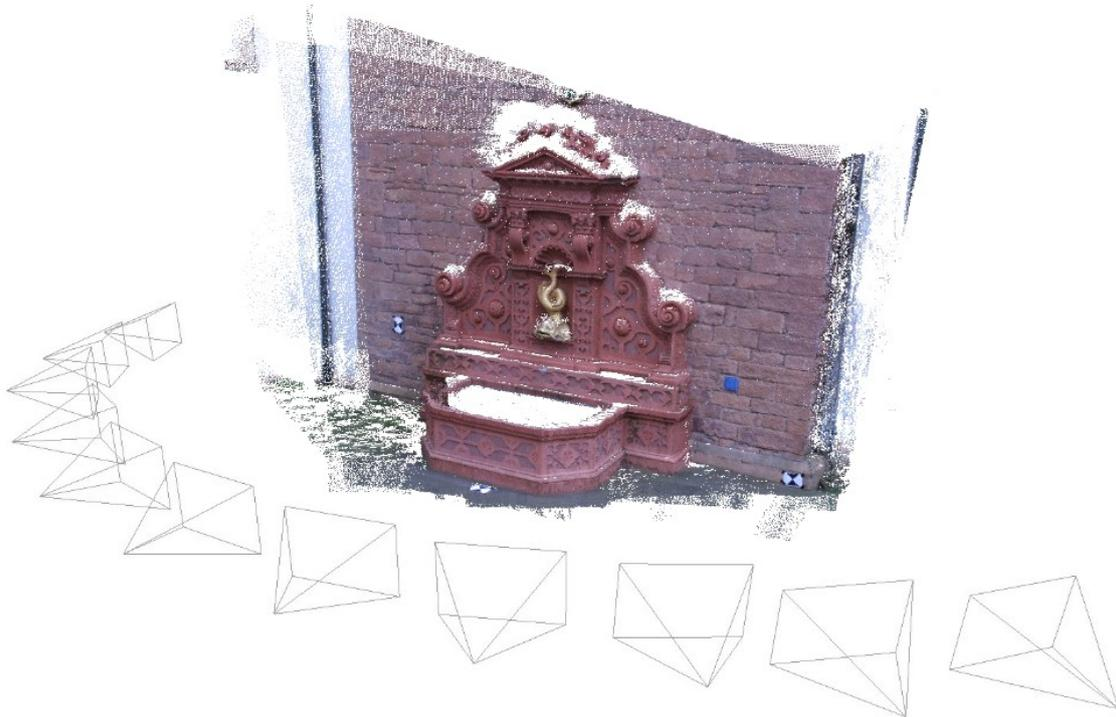
Figure 5.10: **3D Point Cloud Reconstruction fountain-P11:** 3D reconstruction as colored point clouds for the complete image sequence of the fountain-P11 datasets. The picture demonstrates the camera setup reconstructed from SfM.
