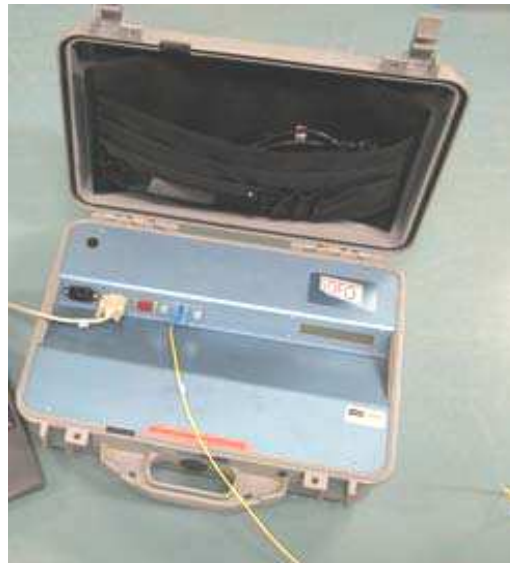
Abbildung B.1: SOFO Static Reading Unit
