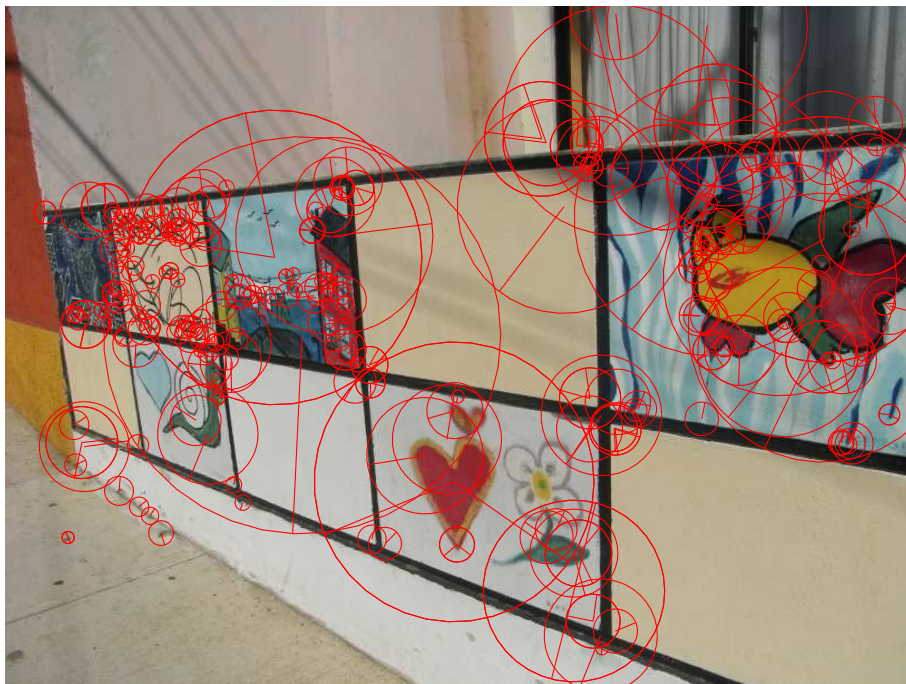
Figure 2.5: The 816 \times 612 image shows about 300 extracted SIFT features. The circles represent the scales of the SIFT features. The radii represent their orientations. Note: There are SIFT keypoints where more than one orientation is assigned at the same scale and location.
