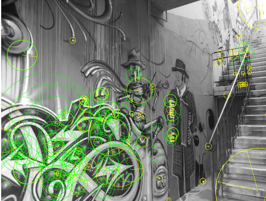
Figure 2.9: The 816 \times 612 image shows about 120 detected SIFT (yellow) and SURF (green) features each. Features are detected at different scales and with different orientations.
