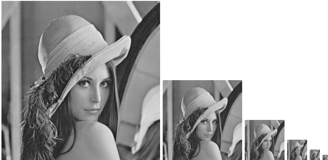
Figure 2.21: First six levels of a Gaussian pyramid. Each higher level is down-scaled by a factor of 2 the dimensions of its predecessor. The size of the original image is 512 \times 512 . The last level has a dimension of 16 \times 16 .
