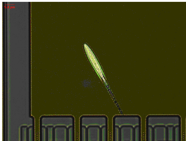
Figure 6.1: Arcing on a wafer surface as occurred during a CVD process.
