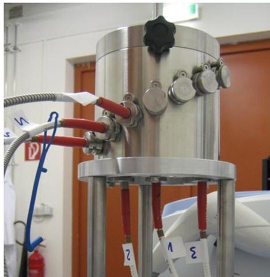
**Figure 5.1.:** NIR-vessel with optical fibres attached.
