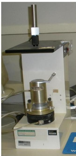
**Figure 2.12.:** A rotational shear cell
