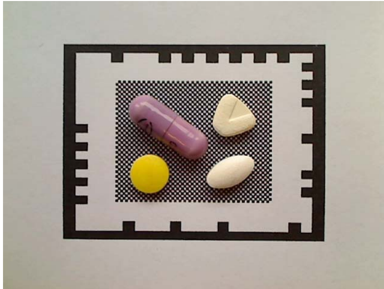
Figure 14: Pills on a frame marker with structured background (square length 0.6 mm, 640 x 480 pixels)
