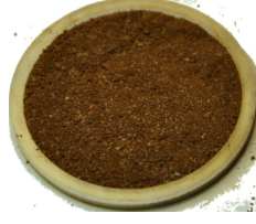
Figure 7.7: To measure liquid and fine granular samples, a silica ring was glued on to the lower electrode plate of the reference instrument.
