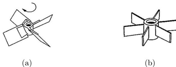
Figure 2.17.: (a) Axial flow impeller: pitched blade turbine and (b) radial flow impeller: open flat blade [26].
