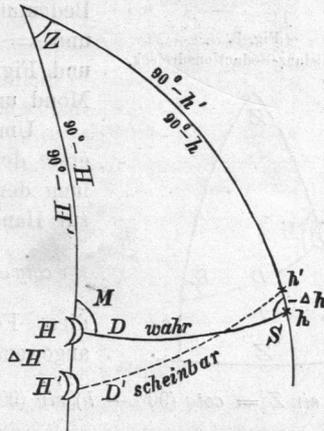
$$\begin{aligned} \cos D &= \cos(90^\circ - H) \cos(90^\circ - h) + \sin(90^\circ - H) \sin(90^\circ - h) \cos Z \\ \cos D' &= \cos(90^\circ - H') \cos(90^\circ - h') + \sin(90^\circ - H') \sin(90^\circ - h') \cos Z \end{aligned}$$
