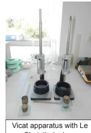
Vicat apparatus with Le Chatelier's rings
