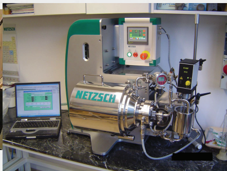
Figure 5. Netzsch MiniCer nano-mill, x_{90} = 100...200 nm
