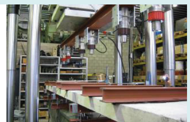
Testing equipment to investigate mechanical properties of construction materials and structural components such as concrete elements and steel profiles (compression test up to 5000kN, tension, bending bench)
