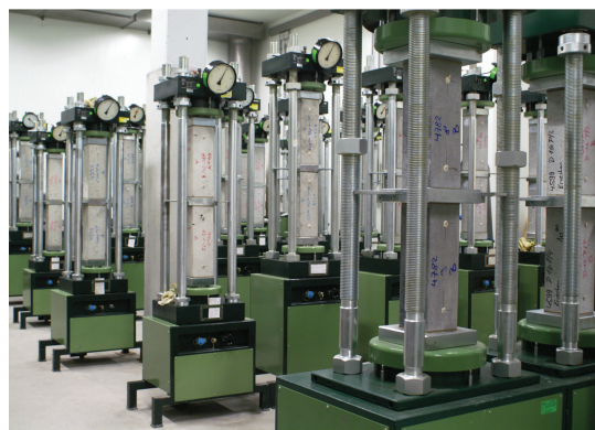
Figure 6: Creep stands for loads up to 600 kN
