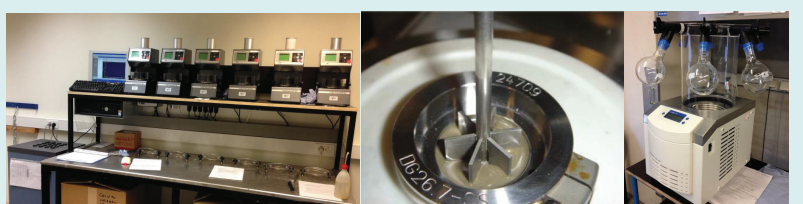
Cement laboratory equipped with isothermal calorimetry, automatic vicat, autogeneous shrinkage dilatometer, viscometer, rheometer and freeze dryer
