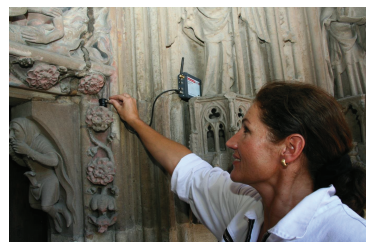
Using wireless sensor nodes for monitoring historical buildings.
