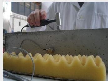
Assessment of dynamical properties such as dynamic modulus of elasticity using modal analysis or ultrasonic pulse method
