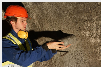
Extracting the core sample and adjusting it to the standard size for further expertise
