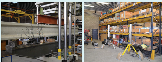
Advanced optical measurement techniques to assess the displacements and deformations during the loading of prestressed concrete beam
