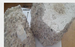
MMCC sensor embedded in concrete sample
