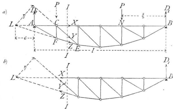
$$0 = Y \eta - D_0 c, \text{ woraus } Y = \frac{D_0 c}{\eta} = \frac{P \xi c}{l \eta} \dots 242.$$
