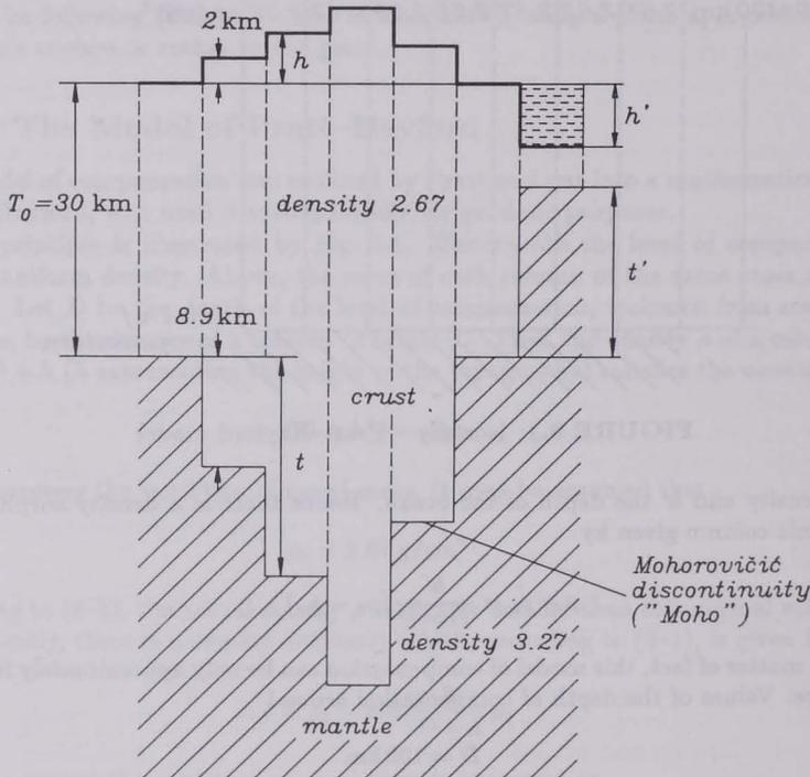
FIGURE 8.2: Isostasy - Airy-Heiskanen model
