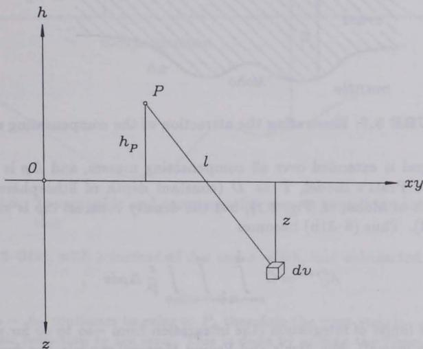
FIGURE 8.6: The basic coordinate systems  $xyz$  and  $xyh$
