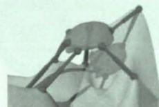
Abb. 4 Parallelmanipulator
