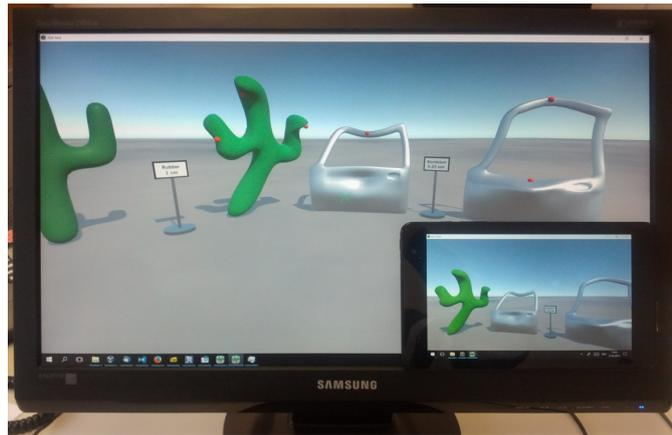
Figure 5.3: Soft-body deformations are synchronized across multiple devices. Both the workstation and the tablet run the same application connected to the simulation web service. Deformations caused by user interaction are immediately synchronized between both devices.
