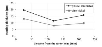
*Figure 3.11:* Distribution of coating thickness along the screw thread for varying protective measures; according to Toblier (2016)
