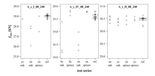
*Figure 3.83:* Steel tensile capacities of screw products A\_s\_I\_08\_240, A\_s\_IV\_08\_240 and A\_s\_II\_08\_240 in dependence of parameter variation
