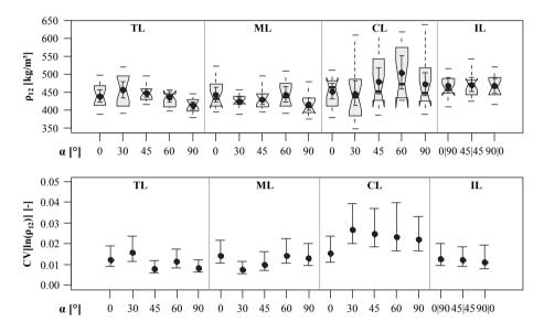
*Figure 5.91:* Above: boxplot graphic of densities  $\rho_{12}$ ; below: CIs of  $CV[ln(\rho_{12})]$ ; test programme I, d = 8 mm;
