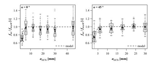
*Figure B.53:* Comparison of test results with model predictions for  $a_{1,CG}$  and  $\alpha = \{0, 45\}^\circ$ ; test data from *Gatternig (2010)*
