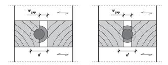
Figure 6.4: Left: screw position leading to the worst case value of  $C_{red}$  determined by Brandner (2016); right: central gap insertion experimentally investigated in section 5-3.4
