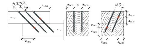
Figure 2.11: Minimum distances of predominately axially loaded screws according to ON EN 1995-1-1 (2015)
