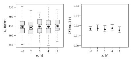
*Figure 5.71:* Left: boxplot diagram of densities  $\rho_{12}$ ; right: CIs of  $CV[ln(\rho_{12})]$  in dependence of spacing  $a_2$ ; test data from Plieschounig (2010);
