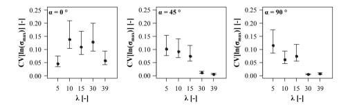
*Figure B.69:* CIs of  $CV[ln(\sigma_{max})]$  in dependence of axis-to-grain angle and slenderness; test specimen corresponding to section 5-4.5
