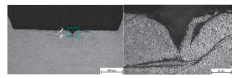
*Figure 3.51:* Further micrographs (etched) of a self-tapping screw's threaded part related to product group A\_s\_II\_08\_240
