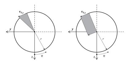
*Figure 3.32:* Comparison of torsional shear stress distributions due to uniform torsion for a circular crosssection; left: stress state (1); right: stress state (III)
