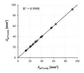
Figure 3.31: Comparison of empirically and numerically determined values of  $A_{pl,N}$
