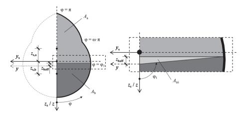
Figure 3.25:Extract and illustration of the triangular area with  $A = A_{tri}$  to be considered for numerical<br/>determination of cross-sectional properties  $z_{half}$  and  $z_{s.(a,b)}$  of the given screw thread profile
