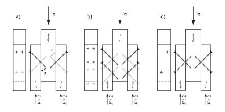
*Figure 2.29:* Screw configurations tested by Tomasi et al. (2010); a) single row and b) double row (a<sub>1</sub> varied) joint with tensioned or compressed screws, c) joint with crossed screws
