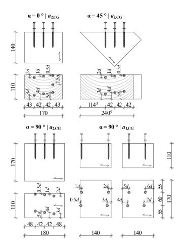
*Figure B.46:* Illustration of test specimen corresponding to section 5-4.1, according to Gatternig (2010); all dimensions in [mm]
