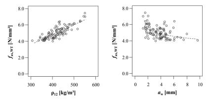
Figure 5.23: Comparison of selected withdrawal and clear wood properties for tangential screw axis orientation
