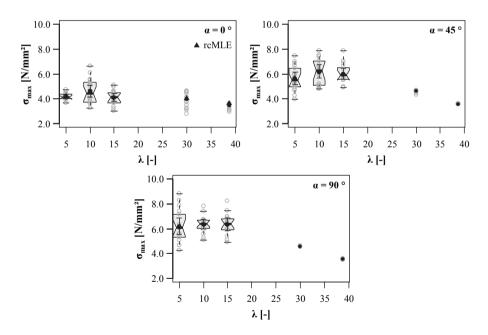
*Figure 5.112:* Combined boxplot/scatterplot graphics of maximum axial stresses reached in dependence of slenderness and axis-to-grain angle
