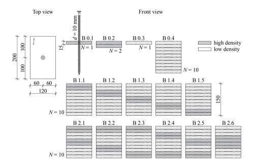
Figure B.25: Illustration of test specimen corresponding to section 5-3.3, test series B; all dimensions in [mm]
