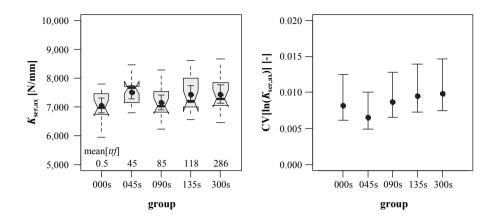
*Figure 5.125:* Left: boxplot graphic of withdrawal stiffness  $K_{ser,ax}$ ; right: CIs of  $CV[ln(K_{ser,ax})]$ , both in dependence of time-to-failure (ttf)
