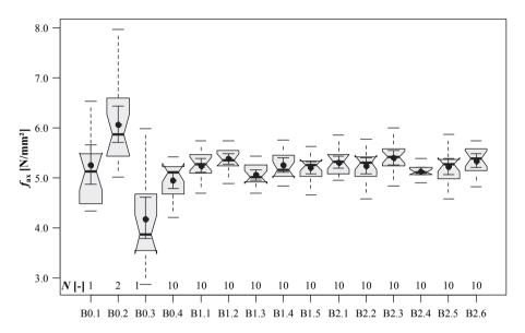
*Figure 5.48:* Boxplot diagrams of withdrawal strength vs. N in dependence of the specific GLT lay-up; test series B
