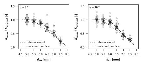
Figure 5.89: Comparison of test results with model predictions for withdrawal stiffness at varying  $d_{PD}$ , d = 8 mm
