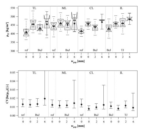
*Figure 5.54:* Above: boxplot graphic of densities  $\rho_{12}$ ; below: CIs of  $CV[ln(\rho_{12})]$  in dependence of gap type and width; test programme I, d = 12 mm
