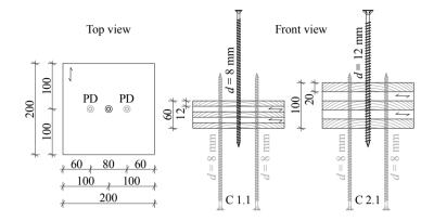
Figure B.26: Illustration of test specimen corresponding to section 5-3.3, test series C; all dimensions in [mm]
