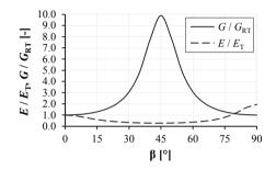
Figure 5.106: Behaviour of apparent elastic material properties E and G in dependence of  $\beta$
