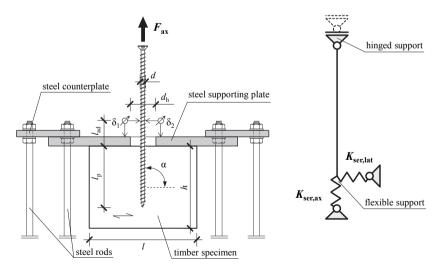
*Figure 5.4:* Screw withdrawal test according to ON EN 1382 (1999); left: schematic illustration of the pushpull test configuration; right: static system with a load application in form of support movement
