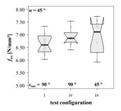
**Figure 5.122:** Withdrawal strength in dependence of test configuration and surface angle  $\varepsilon_{sur}$ ; according to Ringhofer and Schickhofer (2014a)
