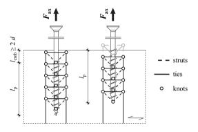
Figure 5.115: Explanation of the "embedment effect" in case of perpendicular-to-grain insertion by means of a strut-and-tie model according to Pirnbacher et al. (2009); left: embedded screw with sufficient  $l_{emb}$ , right: non-embedded screw with  $l_{emb} = 0$  mm
