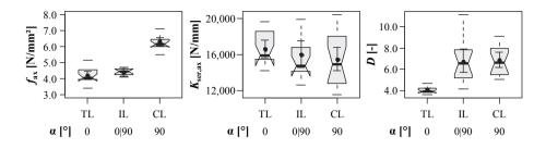
*Figure 5.97:* Boxplot diagrams of screw withdrawal properties when situated in intermediate layers; test data from Grabner (2013); d = 8 mm,  $\alpha = 0|90^{\circ}$
