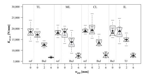
*Figure 5.57:* Boxplot diagrams of withdrawal stiffness vs.  $w_{gap}$  in dependence of screw position and gap type; test programme I, d = 8 mm
