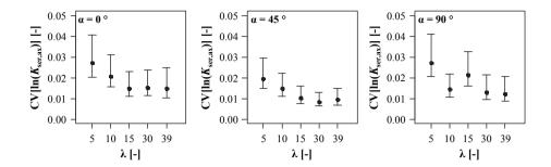
*Figure B.70:* CIs of CV[ln(K<sub>ser,ax</sub>)] in dependence of axis-to-grain angle and slenderness; test specimen corresponding to section 5-4.5
