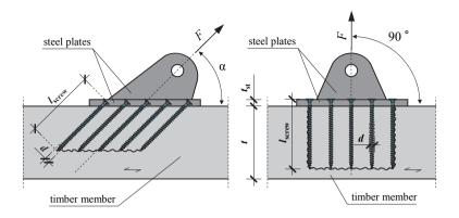
*Figure 2.35:* Crack formation (block shear failure) of inclined steel-to-timber joints; left: general definition with varying  $\alpha$ ; right: worst case scenario at  $\alpha = 90^{\circ}$
