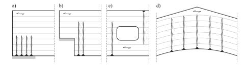
Figure 2.5: Fully threaded self-tapping screws applied as beam reinforcements; according to Blaβ and Bejtka (2004a); a) compression perpendicular to grain at supporting; b) tension perpendicular to grain at notched supporting; c) tension perpendicular to grain at hole; d) tension perpendicular to grain in apex area
