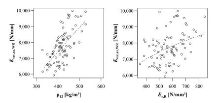
Figure 5.21: Comparison of selected withdrawal and clear wood properties for radial screw axis orientation (continued)
