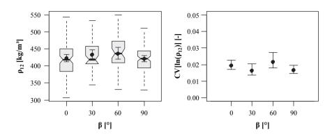
*Figure 5.107:* Left: boxplot graphic of densities  $\rho_{12}$ ; right: CIs of  $CV[ln(\rho_{12})]$ , both in dependence of annual ring orientation
