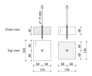
*Figure B.55:* Illustration of test specimen corresponding to section 5-4.2; left:  $\alpha = 90^\circ$ , right:  $\alpha = 0^\circ$ ; all dimensions in [mm]
