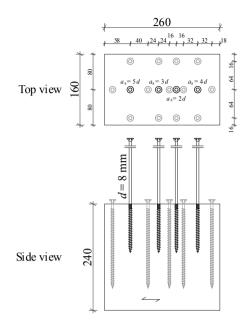
*Figure B.74:* Illustration of test specimen corresponding to section 5-5.1, variation of the supporting screw's  $a_s$ ; all dimensions in [mm]
