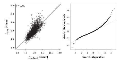
Figure 6.5: Left: experimentally determined vs. predicted reference withdrawal strength  $f_{ax}$  for perpendicular-to-grain insertion in solid timber; right: qq-residual plot
