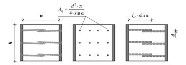
*Figure 2.34:* Different possibilities of determining the reduced cross-sectional area; left: cross-section of the screwed connection; middle: cut surfaces of screw axis; right: projection of screws' outer thread surfaces; according to Ringhofer et al. (2014b)
