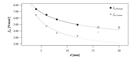
*Figure 5.12:* Comparison of experimentally determined withdrawal strength with model prediction at varying outer thread diameter d
