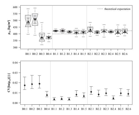
*Figure 5.41:* Above: boxplot graphic of densities  $\rho_{12}$ ; below: CIs of  $CV[[n(\rho_{12})]$  in dependence of the specific GLT lay-up; series B
