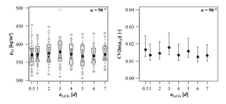
*Figure 5.69:* Left: combined boxplot/scatterplot graphic of densities  $\rho_{12}$ ; right: CIs of  $CV[ln(\rho_{12})]$  in dependence of spacing  $a_{1,CG}$  for axis-to-grain angle  $\alpha = 90^\circ$ ; test data from Gatternig (2010)
