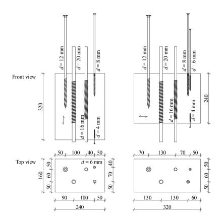
*Figure B.15:* Illustration of test specimen corresponding to section 5-2.1; left:  $\alpha = 0^\circ$ , right:  $\alpha = 90^\circ$ ; all dimensions in [mm]
