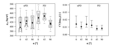
*Figure 5.78:* Left: boxplot diagram of densities  $\rho_{12}$ ; right: CIs of  $CV[[n(\rho_{12})]$  in dependence of pre-drilling and axis-to-grain angle  $\alpha$ ; test data from Grabner (2013);
