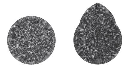
Figure 3.17: FE-meshes generated by the software package written by Bogensperger (2002); left: inner thread cylinder,  $d_c = 5.2$  mm; right: screw thread cross-section if {d, p, v, η} = {8.0 mm, 3.8 mm, 40 °, 0.65}
