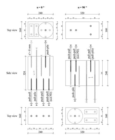
*Figure B.72:* Illustration of test specimen corresponding to section 5-5.1, variation of test configurations; all dimensions in [mm]
