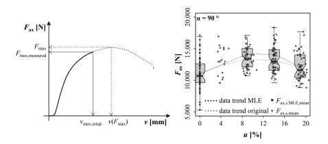
**Figure 5.34:** Left: measurement error of withdrawal capacity in the force-displacement relationship; right: comparison of results from Pirnbacher et al. (2009) with corrected values (ST,  $\alpha = 90^{\circ}$ ); both according to Ringhofer et al. (2014c)
