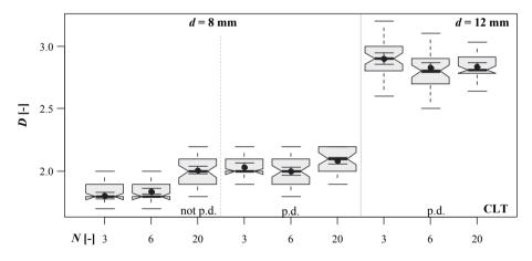
Figure 5.47: Boxplot diagrams of ductility vs. N in dependence of d and pre-drilling; test series A, CLT
