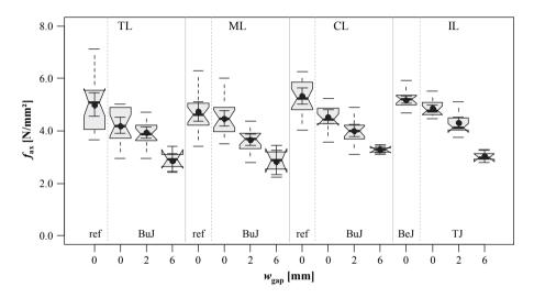
*Figure 5.59:* Boxplot diagrams of withdrawal strength vs.  $w_{gap}$  in dependence of screw position and gap type; test programme I, d = 12 mm
