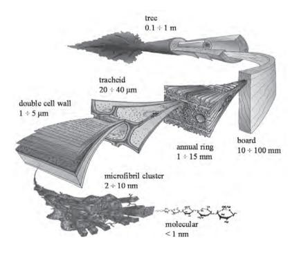
Figure 4.1: Schematic overview of the structural hierarchy of softwood; according to Harrington (2002)
