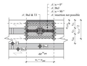
*Figure 6.3:* Definition of gap types and illustration of areas related to different axis-to-grain directions and gap types exemplarily for screw insertion normal to the CLT narrow face; according to Ringhofer et al. (2015c)
