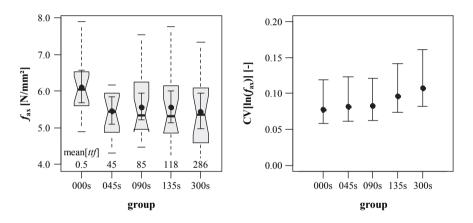
**Figure 5.124:** Left: boxplot graphic of withdrawal strength  $f_{ax}$ ; right: CIs of  $CV[ln(f_{ax})]$ , both in dependence of time-to-failure (ttf)
