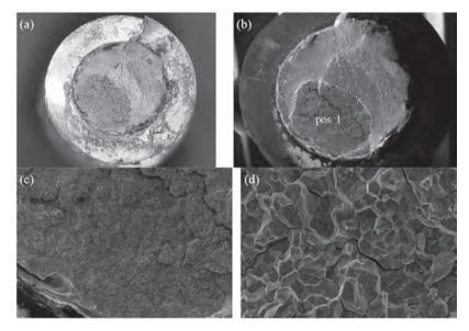
*Figure 3.89:* A\_s\_II\_08\_240 (yc) in oak; (a) fracture pattern; (b) SEM scan with zoom positions; (c) and (d) zoom view of pos. 1; 50x/1000x magnification; according to Toblier (2016)
