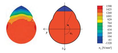
*Figure 3.42:* Comparison of analytically (middle) and numerically (left) determined normal stress distributions at the screw thread profile in case of  $N = N_{pl}$  and  $\{d, \eta, v, p\} = \{8.00 \text{ mm}, 0.65, 40^\circ, 3.80 \text{ mm}\}$
