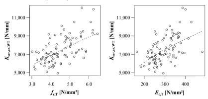
*Figure 5.27:* Comparison of selected withdrawal and clear wood properties for tangential screw axis orientation (continued)
