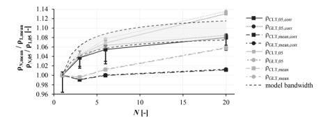
*Figure 5.39:* Corrected and uncorrected behaviour of timber density in dependence of N for density group 1G; according to Ringhofer et al. (2015b)
