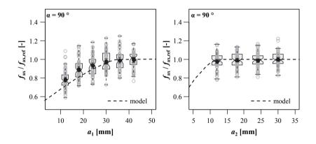
*Figure B.54:* Comparison of test results with model predictions for  $a_1$  and  $a_2$  at  $\alpha = 90^\circ$ ; test data from *Plieschounig (2010)*
