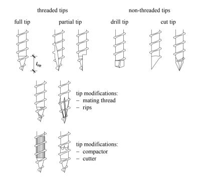
Figure 3.6: Classification and geometrical parameters of screw tips
