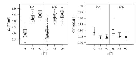
*Figure 5.81:* Left: boxplot diagram of withdrawal strength  $f_{ax}$ ; right: CIs of  $CV[ln(f_{ax})]$ ; both in dependence of axis-to-grain angle and pre-drilling, test data from Grabner (2013);
