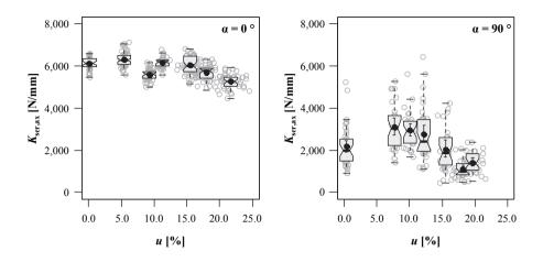
*Figure 5.31:* Combined boxplot/scatterplot diagrams of withdrawal stiffness vs. moisture content; left:  $\alpha = 0$ °; right:  $\alpha = 90$ °; experimental campaign I
