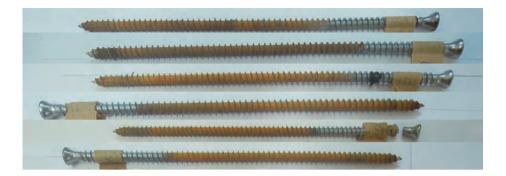
Figure B.12: Macrophotos of A\_s\_II\_08\_240 (zinc-nickel) applied in oak; test campaign II
