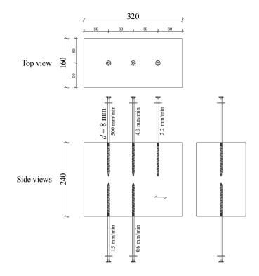
Figure B.78: Illustration of test specimen corresponding to section 5-5.2; all dimensions in [mm]
