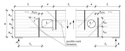
*Figure 2.47:* Different types of holes in timber members reinforced with self-tapping screws: left: prismatic hole; right: round hole
