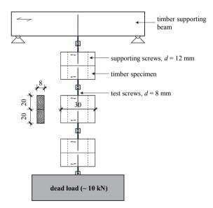
Figure 3.73: Schematic illustration of the long-term test configuration; dimensions in [cm]
