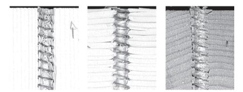
Figure 5.2: Photographs of cut views made for the observation of withdrawal failure; left: LT-plane; middle: RL-plane; right: RT-plane
