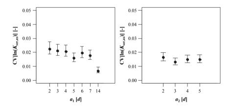
*Figure B.50:* CIs of  $CV[ln(K_{ser,ax})]$  in dependence of spacing type  $a_1$  and  $a_2$ ; test specimen corresponding to section 5-4.1, test data from Plieschounig (2010)
