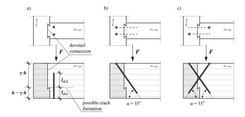
Figure 2.46: Dovetail joints reinforced with self-tapping screws according to Tannert and Lam (2009); a) reinforcement equal to notched timber beams, b) and c) reinforcement with inclined screws, similar to a transversal joint
