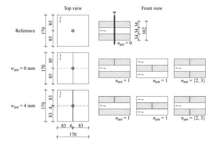
*Figure B.35:* Illustration of test specimen corresponding to section 5-3.4, test campaign II; all dimensions in [mm]
