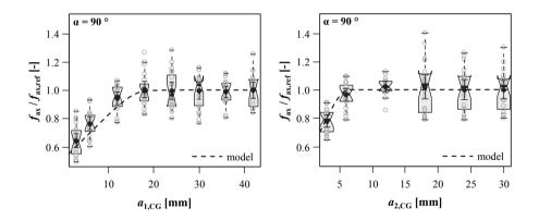
*Figure B.52:* Comparison of test results with model predictions for  $a_{1,CG}$  and  $a_{2,CG}$  at  $\alpha = 90$ °; test data from *Gatternig (2010)*
