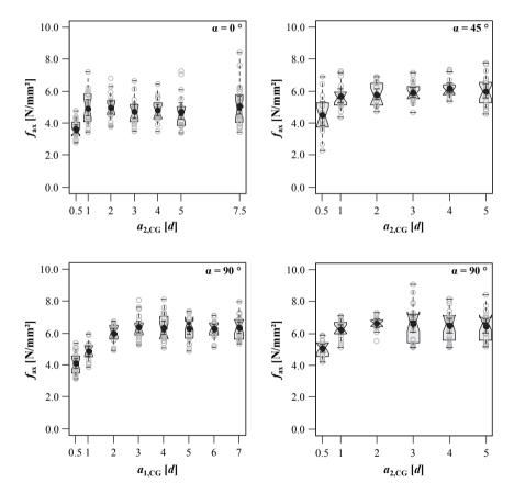
Figure 5.72: Combined boxplot/scatterplot diagrams of withdrawal strength vs.  $a_{1,CG}$  and  $a_{2,CG}$ in dependence of a; test data from Gatternig (2010)
