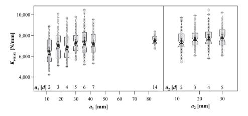
*Figure 5.74:* Combined boxplot/scatterplot diagram of withdrawal stiffness vs. spacing  $a_1$  and  $a_2$ ; test data from Plieschounig (2010)
