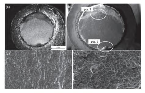
*Figure 3.66:* SEM images of a screw failed at N = 2,088,700; (a) photo of the fracture pattern; (b) microscopic scan with zoom positions; (c) zoom view of pos. 1; (d) zoom view of pos. 2; 500x magnification
