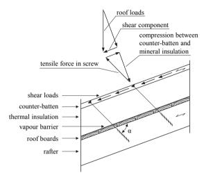
Figure 2.3: Fastening of thermal insulation material on top of rafters – detail and loadbearing model; according to Blaβ (2000b) and ETA-11/0190 (2013)
