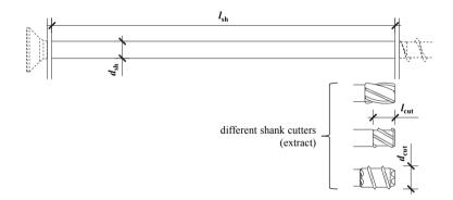
Figure 3.4: Geometrical parameters of screw shanks, including an extract of cutter geometries
