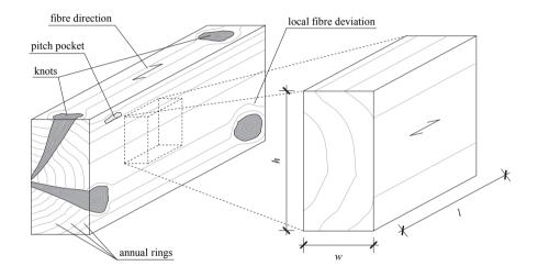
Figure 4.2: Definition of clear wood specimen applied for investigations on self-tapping screws
