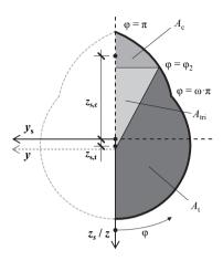
**Figure 3.29:** Illustration of the triangular area with  $A = A_{tri}$  to be considered for numerical determination of cross-sectional properties  $\varphi_2$ ,  $A_{(c,t)}$  and  $z_{s,(c,t)}$  of the given screw thread profile
