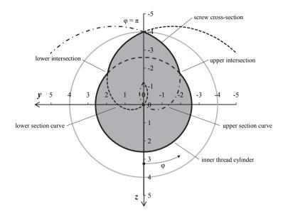
*Figure 3.15:* Cross-sectional shape of an example screw's threaded part at x = p/2
