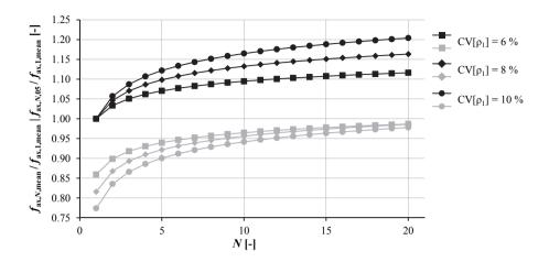
*Figure 5.37:* Behaviour of mean (black) and 5 %-quantile (grey) values of  $f_{ax,N}/f_{ax,1}$  in dependence of N and  $CV[\rho_1]$  for  $k_{CV} = 1.5$ ; according to Ringhofer et al. (2015b)
