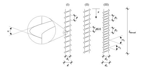
Figure 3.5: Classification and geometrical parameters of screw threads
