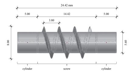
Figure 3.40: 3D full scale model of one example screw generated by the software package RFEM 5 (2012)
