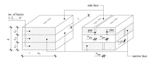
Figure 4.7: Relevant characteristics of unidirectional and orthogonal layered clear wood
