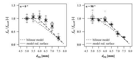
*Figure 5.88:* Comparison of test results with model predictions for withdrawal strength at varying  $d_{PD}$ , d = 8 mm
