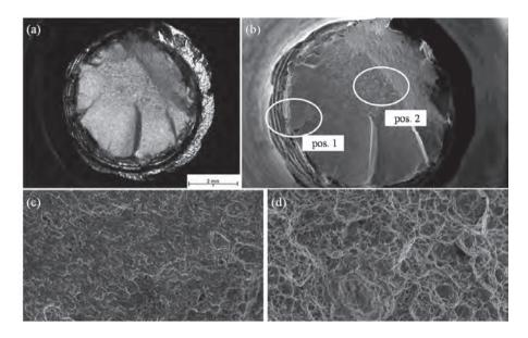
Figure 3.65:SEM images of a screw failed at N = 144,500; (a) photo of the fracture pattern; (b) microscopic<br/>scan with zoom positions; (c) zoom view of pos. 1; (d) zoom view of pos. 2; 500x magnification
