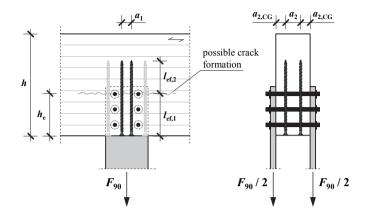
*Figure 2.44:* Dowel-type connection with a force component perpendicular to grain reinforced with self-tapping screws
