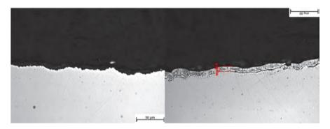
*Figure 3.80:* Comparison of corrosion in oak (left) and Norway spruce (right); sample A\_s\_1\_08\_240 (zincnickel coating) as part of test campaign I; according to Hauptmann (2016)
