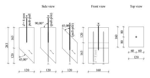
**Figure B.75:** Illustration of test specimen corresponding to section 5-5.1, variation of test configurations and surface angle  $\varepsilon_{sur}$ ; all dimensions in [mm]
