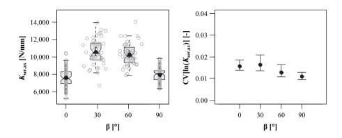
Figure 5.109: Left: combined boxplot/scatterplot graphic of density corrected withdrawal stiffness  $K_{ser,ax}$ , right: CIs of  $CV[ln(K_{ser,ax})]$ , both in dependence of annual ring orientation
