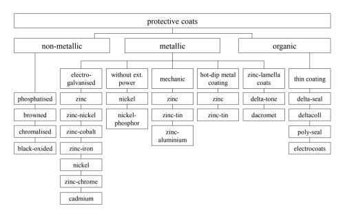
*Figure 3.10:* Overview and classification of protective coats applied for screw production; according to ABC-Verbindungsmittel (2008)
