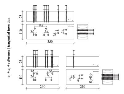
*Figure B.45:* Illustration of test specimen corresponding to section 5-4.1, according to Plieschounig (2010) (continued); all dimensions in [mm]
