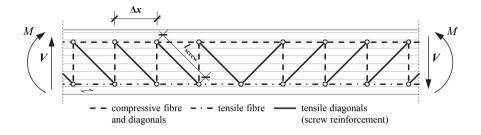
Figure 2.49: Example of a truss-like screw arrangement in GLT beams stressed in bending; according to Trautz and Koj (2009)
