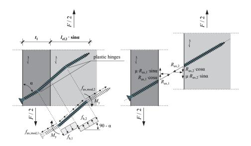
Figure 2.28: Left: schematic illustration of forces and stress distributions in an inclined screwed timber-totimber connection for Johansen's failure mode 3; according to Blaβ and Bejtka (2001) and Bejtka and Blaβ (2002); right: truss-like force system exclusively considering axial screw capacity; according to Blaβ and Bejtka (2003b)
