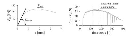
*Figure 5.6:* Left: typical test curve of an axially loaded screw; right: load increment vs. time step of this test curve, determined in accordance to Brandner et al. (2017)
