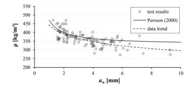
Figure 4.4: Comparison of the approach according to Persson (2000) with own test results
