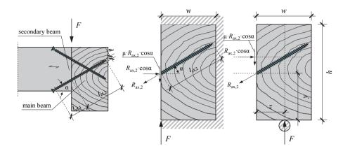
*Figure 2.36:* Left: main to secondary beam transversal joint with crossed screws; middle: force system at fixedend main beam; right: force system at hinged supported main beam; according to Blaβ and Bejtka (2003b)
