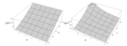
*Figure 3.48:* Influence of thread properties on plastic area  $A_{pl,N}$  for d = 8 mm; left:  $v = 40^\circ$ ; right:  $\eta = 0.65$
