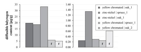
*Figure 3.92:* Diffusible hydrogen contents of five samples A\_s\_II\_08\_240, applied in oak and spruce, test campaign II (f = failed screws): left: protective coating, right: steel
