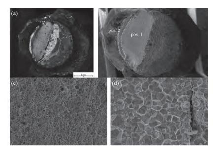
*Figure 3.88:* A\_s\_1\_08\_240 (zn) in oak; (a) fracture pattern; (b) SEM scan with zoom positions; (c) zoom view of pos. 1 (500x); (d) zoom view of pos. 2 (1000x magnification); according to Hauptmann (2016)
