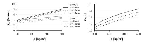
**Figure 5.13:** Left: withdrawal strength  $f_{ax}$  vs. density  $\rho$ ; right: ratios  $k_{90}$  vs. density  $\rho$ ; both in dependence of  $\alpha$  and d; predicted according to Pirnbacher et al. (2009)
