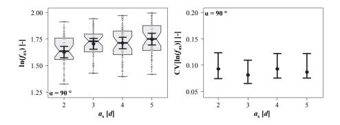
*Figure 5.121:* Left: logarithmic withdrawal strength, right: CIs of  $CV[ln(f_{ax})]$ , both in dependence of the supporting screws' distance  $a_s$ ; according to Ringhofer and Schickhofer (2014a)
