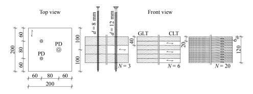
Figure B.24: Illustration of test specimen corresponding to section 5-3.3, test series A; all dimensions in [mm]
