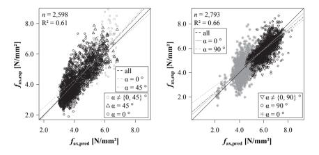
**Figure 6.7:** Experimentally determined vs. predicted withdrawal strength  $f_{ax}$ ; left: tests with solid timber at  $\alpha \neq 90^{\circ}$ ; right: tests with GLT and CLT according to Ringhofer et al. (2015a)
