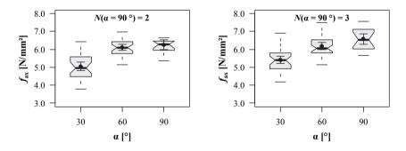
*Figure 5.103:* Boxplot diagram of screw withdrawal strength  $f_{ax}$  in dependence of  $N(\alpha = 90^{\circ})$  and axis-to-grain angle, d = 8 mm; test programme II
