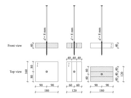
*Figure B.17:* Illustration of withdrawal test specimen corresponding to section 5-3.1; from left to right: radial, tangential, longitudinal direction; all dimensions in [mm]
