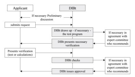
Figure 2.15: Procedure for obtaining a National Technical Approval, according to DIBt (2015d)
