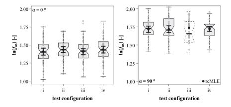
Figure 5.119: Logarithmic withdrawal strength in dependence of axis-to-grain angle and test configuration; according to Ringhofer and Schickhofer (2014a)
