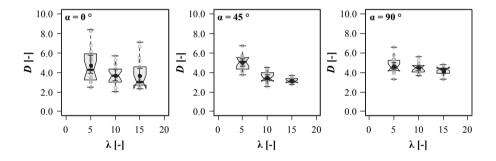
*Figure 5.114:* Combined boxplot/scatterplot graphics of ductility D in dependence of slenderness and axis-tograin angle
