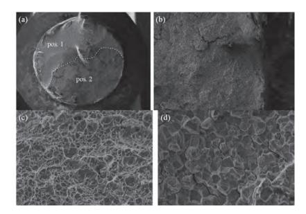
*Figure 3.90:* A\_s\_II\_08\_240 (yc) in Norway spruce; (a) SEM scan with zoom positions; (c) zoom view of pos. 1; 1000x magnification; (b) and (d) zoom view of pos. 2; 50x/1000x magnification; according to Toblier (2016)
