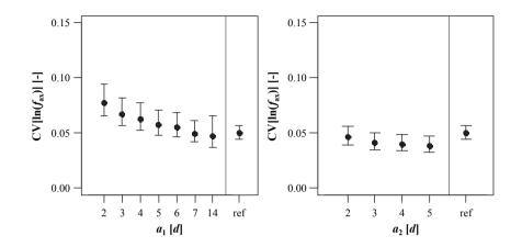
**Figure B.49:** CIs of  $CV[ln(f_{ax})]$  in dependence of spacing type  $a_1$  and  $a_2$ ; test specimen corresponding to section 5-4.1, test data from Plieschounig (2010)
