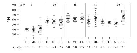
*Figure 5.96:* Boxplot diagram of ductility D in dependence of axis-to-grain angle and ratio  $t_l / d$ ; test data from Grabner (2013); d = 8 mm
