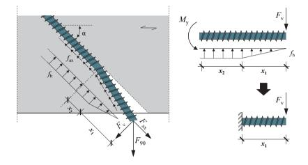
Figure 2.31: Left: schematic illustration of forces and stress distributions in an inclined screwed timber-totimber connection loaded perpendicular to grain; right: stiffness model simplification with reduced embedment strength; according to Jockwer et al. (2014)
