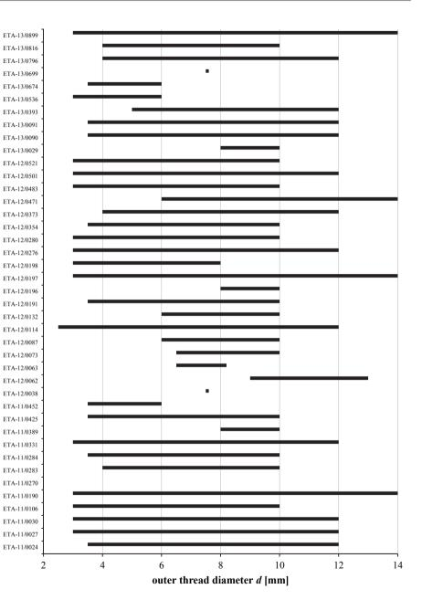
Figure B.2: Overview of the outer thread diameter bandwidth of all ETAs analysed
