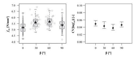
**Figure 5.108:** Left: combined boxplot/scatterplot graphic of density corrected withdrawal strengths  $f_{ax}$ ; right: CIs of  $CV[ln(f_{ax})]$ , both in dependence of annual ring orientation
