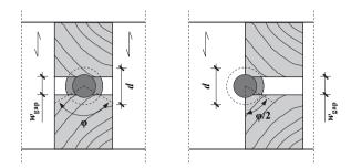
Figure 5.51: Screw insertion in gaps of CLT narrow face; left: BuJ; right: TJ
