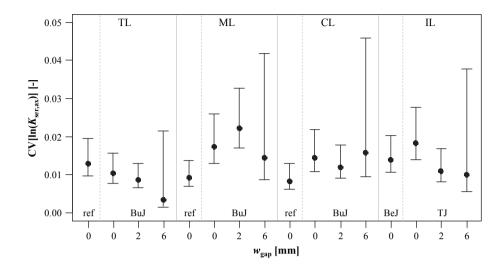
*Figure B.37:* CIs of  $CV[ln(K_{ser,ax})]$ ; test programme I, d = 8 mm; test specimen corresponding to section 5-3.4
