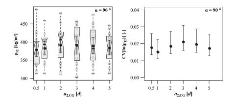
**Figure 5.68:** Left: combined boxplot/scatterplot graphic of densities  $\rho_{12}$ ; right: CIs of  $CV[ln(\rho_{12})]$  in dependence of spacing  $a_{2,CG}$  for axis-to-grain angle  $\alpha = 90^\circ$ ; test data from Gatternig (2010)
