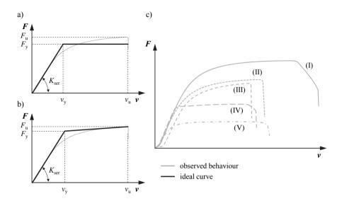
Figure 3.37: Determination of F<sub>y</sub> and D for self-tapping screws loaded in tension; (a) according to ASTM E2126 (2002); (b) according to ON EN 12512 (2001); (c) illustration of five typical test curves observed
