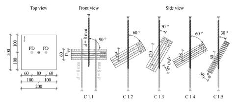
*Figure B.60:* Illustration of test specimen corresponding to section 5-4.3, test campaign II; exemplarily for d = 8 mm; all dimensions in [mm]
