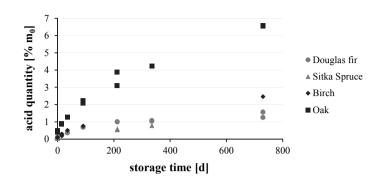
*Figure 3.68:* Quantity of acetic acid in dependence of storage time (days) at T = 48 °C and wet climate (damp conditions) for four timber species; data from Packman (1960)
