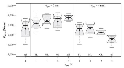
Figure 5.61: Boxplot diagrams of withdrawal stiffness vs. w<sub>gap</sub> and n<sub>gap</sub>; test programme II
