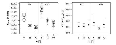
*Figure 5.83:* Left: boxplot diagram of withdrawal stiffness  $K_{ser,ax}$ ; right: CIs of CV[ $ln(K_{ser,ax})$ ]; both in dependence of axis-to-grain angle and pre-drilling, test data from Grabner (2013)
