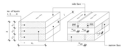
Figure 5.36: Relevant characteristics of unidirectional and orthogonal layered clear wood
