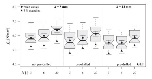
*Figure 5.42:* Boxplot diagrams of withdrawal strength vs. N in dependence of d and pre-drilling; test series A, GLT
