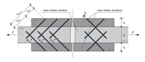
Figure 2.27: Cross-section of a typical timber-to-timber tensile connection with inclined positioned self-tapping screws; left: tensioned screw joint; right: crossed screw joint
