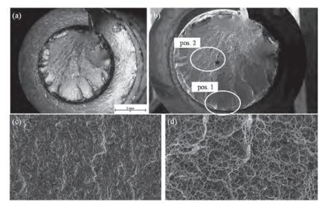
*Figure 3.64:* SEM images of a screw failed at N = 31,500; (a) photo of the fracture pattern; (b) microscopic scan with zoom positions; (c) zoom view of pos. 1; (d) zoom view of pos. 2; 500x magnification
