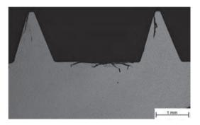
*Figure 3.50:* Micrograph (etched) of a self-tapping screw's threaded part related to product group A\_s\_II\_08\_240
