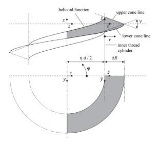
Figure 3.13: Illustration of mathematical functions describing the three-dimensional screw thread profile
