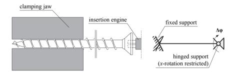
*Figure 3.38:* Screw torsional test according to ON EN 14592 (2012); left: schematic illustration of the test set-up; right: static system with load application in form of support rotation
