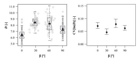
*Figure 5.110:* Left: combined boxplot/scatterplot graphic of ductility D; right: CIs of CV[ln(D)], both in dependence of annual ring orientation
