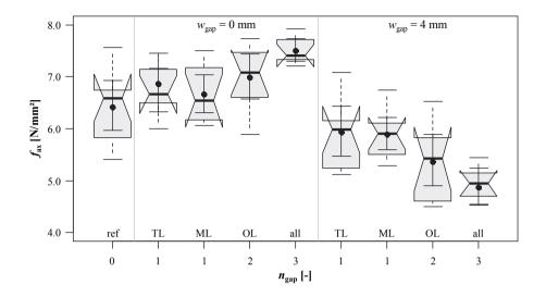
Figure 5.60: Boxplot diagrams of withdrawal strength vs. w<sub>gap</sub> and n<sub>gap</sub>; test programme II
