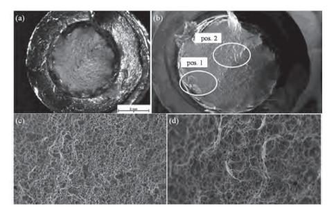
*Figure 3.61:* SEM images of the reference screw ( $N = 10^{0}$ ); (a) photo of the fracture pattern; (b) microscopic scan with zoom positions; (c) zoom view of pos. 1; (d) zoom view of pos. 2; 500x magnification
