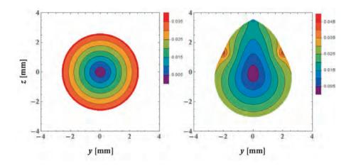
*Figure 3.18:* Shear stress distributions  $[N/mm^2]$  due to uniform torsion ( $M_T = 1 Nmm$ ) determined with the software application from Bogensperger (2002); left: inner thread cylinder,  $d_c = 5.2 mm$ ; right: screw thread cross-section in case of {d, p, v,  $\eta$ } = {8.0 mm, 3.8 mm, 40 °, 0.65}
