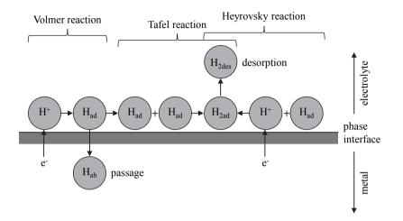
Figure 3.53: Schematic illustration of electrochemical hydrogen discharge; according to Landgrebe (1993)
