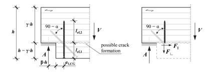
*Figure 2.45:* Left: supporting of a notched timber beam reinforced with self-tapping screws; right: force components parallel and perpendicular to crack formation transferred by the reinforcements, according to Jockwer (2014)
