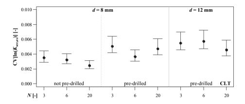
*Figure B.30:* CIs of CV[ln(K<sub>ser,ax</sub>)] in dependence of N, d and pre-drilling; series A, CLT; test specimen corresponding to section 5-3.3
