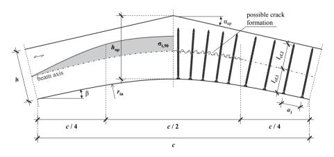
*Figure 2.48:* Tensile stress distribution perpendicular to grain and reinforcement with self-tapping screws of a pitched cambered beam loaded in bending
