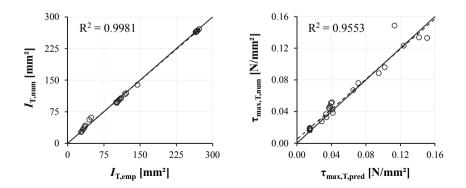
*Figure 3.22:* Comparison of approximated and numerically determined values of  $I_T$  (left) and  $\tau_{max,T}$  (right)
