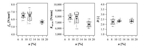
*Figure 5.33:* Combined boxplot/scatterplot diagrams of withdrawal strength (left), stiffness (middle) and ductility (right) vs. moisture content;  $\alpha = 90^\circ$ ; experimental campaign II
