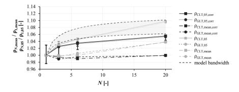
*Figure 5.40:* Corrected and uncorrected behaviour of timber density in dependence of N for density group 2G; according to Ringhofer et al. (2015b)
