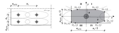
*Figure 5.65:* Left: top view of a screwed connection inserted at  $\alpha = 90^{\circ}$ ; right: definition of the reduced stressable timber volume for the special case of an edge screw
