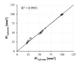
Figure 3.35: Comparison of empirically and numerically determined values of  $W_{T,pl}$
