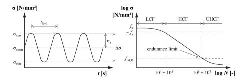
Figure 3.56: Left: load-time relationship of a typical Wöhler fatigue test in the pulsating tensile domain; right: S/N-diagram with classification of different fatigue domains; according to Radaj and Vormwald (2007) and Schäfer (2008)
