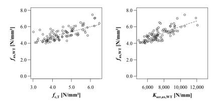
*Figure 5.24:* Comparison of selected withdrawal and clear wood properties for tangential screw axis orientation (continued)
