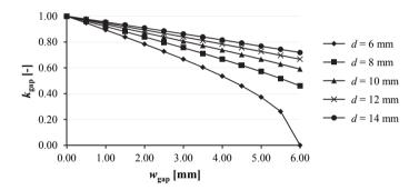
*Figure 5.52:* Behaviour of  $k_{gap}$  for screw insertion in BuJ in dependence of d and  $w_{gap}$  ( $n_{gap} = N = 1$ )
