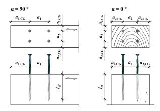
*Figure 5.64:* Definition of minimum spacings according to ON EN 1995-1-1 (2015); left:  $\alpha = 90^\circ$ ; right:  $\alpha = 0^\circ$
