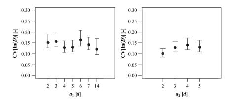
**Figure B.51:** CIs of CV[ln(D)] in dependence of spacing type  $a_1$  and  $a_2$ ; test specimen corresponding to section 5-4.1, test data from Plieschounig (2010)
