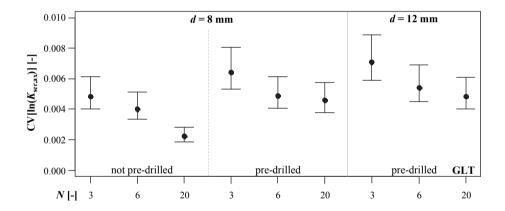
*Figure B.29:* CIs of CV[ln(K<sub>ser,ax</sub>)] in dependence of N, d and pre-drilling; series A, GLT; test specimen corresponding to section 5-3.3
