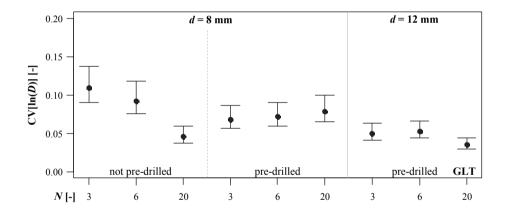
*Figure B.31:* CIs of CV[ln(D)] in dependence of N, d and pre-drilling; series A, GLT; test specimen corresponding to section 5-3.3
