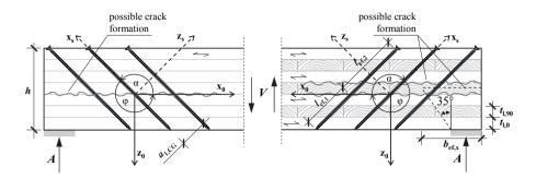
Figure 2.50: Screw reinforcement of laminated timber members against shear stresses, denotation of coordinates and angles within the structural anisotropy: left: GLT; right: CLT; according to Dietsch et al. (2012)
