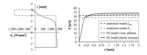
*Figure 3.43:* Left: analytically and numerically determined normal stress distributions at y = 0 and  $N = N_{pl}$ ; right: numerically determined force-displacement curves for the screw thread loaded in tension
