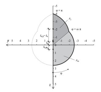
*Figure 3.16:* Partial areas and gravity centre positions for an example screw's threaded part at x = p/2
