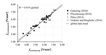
Figure 5.76: Experimental vs. predicted withdrawal strengths regarding the influence of spacings on  $f_{ax}$
