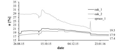
Figure 3.77: Distribution of moisture content recorded in the frame of test campaign II
