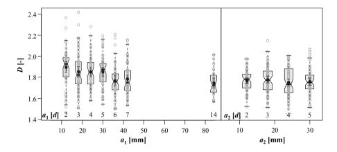
**Figure 5.75:** Combined boxplot/scatterplot diagram of ductility vs. spacing  $a_1$  and  $a_2$ ; test data from Plieschounig (2010)
