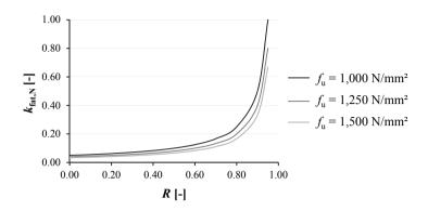
*Figure 3.57:* Behaviour of  $k_{fat,N}$  in dependence of R for varying steel tensile strengths  $f_u$
