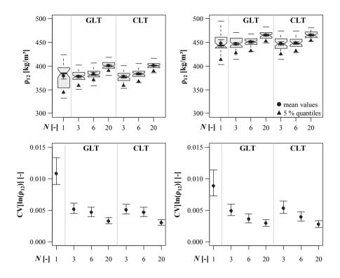
*Figure 5.38:* Above: boxplot graphic of densities  $\rho_{12}$ ; below: CIs of  $CV[\ln(\rho_{12})]$  in dependence of timber product, density group and number of penetrated layers; left: group 1G; right: group 2G; series A
