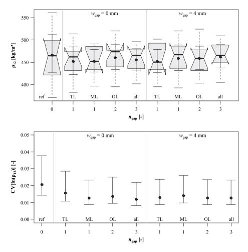
**Figure 5.55:** Above: boxplot graphic of densities  $\rho_{12}$ ; below: CIs of  $CV[ln(\rho_{12})]$  in dependence of  $w_{gap}$  and  $n_{gap}$ ; test programme II
