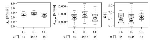
*Figure 5.98:* Boxplot diagrams of screw withdrawal properties when situated in intermediate layers; test data from Grabner (2013); d = 8 mm,  $\alpha = 45|45 \circ$
