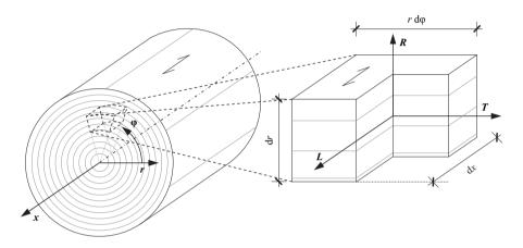
Figure 4.5: Symmetry planes L, R and T of an infinitesimal timber volume element
