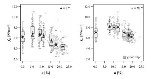
*Figure 5.30:* Combined boxplot/scatterplot diagrams of withdrawal strength vs. moisture content; left:  $\alpha = 0^{\circ}$ ; right:  $\alpha = 90^{\circ}$ ; experimental campaign I
