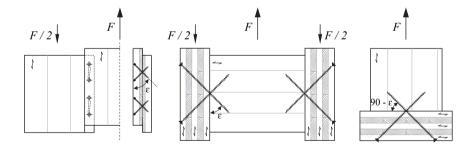
**Figure 2.41:** Different CLT connections with axially loaded crossed screws (exemplarily,  $\varepsilon = 45^{\circ}$ ); left: stepped joint as in-plane connection; middle and right: wall-to-floor joint as out-of-plane connection; according to Bratulic et al. (2014a)
