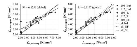
*Figure 5.63:* Experimental vs. predicted withdrawal strengths; left: originally assumed TJ; right: TJ assumed as BuJ
