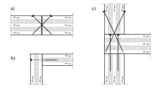
*Figure 2.8: Fully and partially threaded self-tapping screws applied in CLT structures; a) floor-to-floor joint; b) wall-to-wall joint; c) wall-to-floor-to-wall joint according to Bernasconi (2012)*
