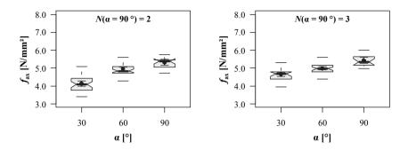
*Figure 5.104:* Boxplot diagram of screw withdrawal strength  $f_{ax}$  in dependence of  $N(\alpha = 90^{\circ})$  and axis-to-grain angle, d = 12 mm; test programme II
