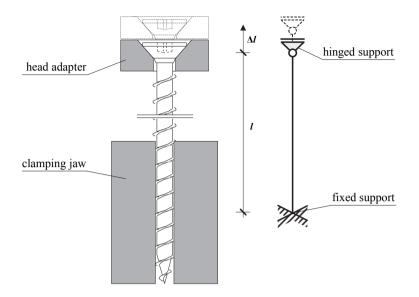
*Figure 3.36:* Screw axial tensile test according to ON EN 14592 (2012); left: schematic illustration of the test set-up; right: static system with load application in form of support movement
