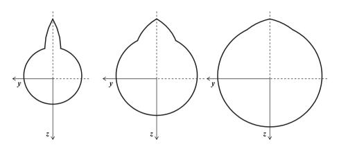
*Figure 3.20:* Illustration of thread cross-sections for three selected parameter sets, d = 8 mm; left: p = 8.0 mm, v = 20 °,  $\eta = 0.50$ ; middle: p = 5.6 mm, v = 40 °,  $\eta = 0.70$ ; right: p = 3.2 mm, v = 60 °,  $\eta = 0.90$
