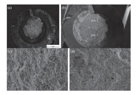
*Figure 3.84:* A\_s\_IV\_08\_240 (bc) in oak; (a) fracture pattern; (b) SEM scan with zoom positions; (c) zoom view of pos. 1; (d) zoom view of pos. 2; 500x magnification; according to Hauptmann (2016)
