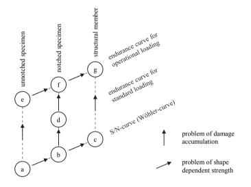
*Figure 3.58:* Classification of fatigue regarding specimen geometry and loading types; according to Haibach (2002)
