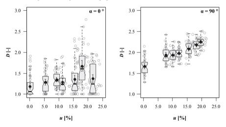
*Figure 5.32:* Combined boxplot/scatterplot diagrams of ductility vs. moisture content; left:  $\alpha = 0^\circ$ ; right:  $\alpha = 90^\circ$ ; experimental campaign I
