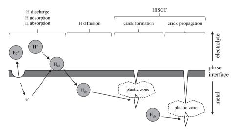
Figure 3.72: Process of HISCC considering decohesion theory; according to Nürnberger (1995)
