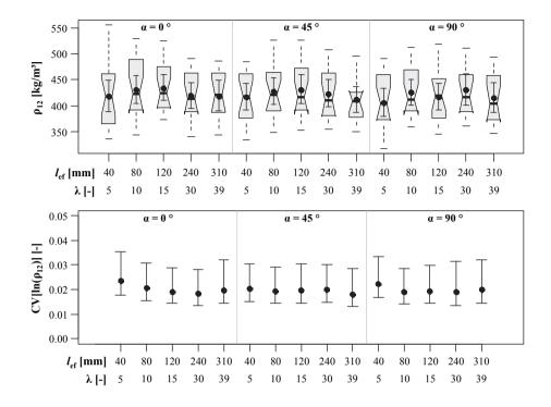
*Figure 5.111:* Above: boxplot graphic of densities  $\rho_{12}$ ; below: CIs of  $CV[ln(\rho_{12})]$ , both in dependence of axis-to-grain angle and effective inserted thread length
