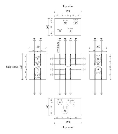
Figure B.73:Illustration of test specimen corresponding to section 5-5.1, variation of the supporting plate's  $d_h$ ;all dimensions in [mm]
