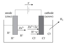
Figure 3.52: Schematic illustration of galvanisation process; according to Toblier (2014)
