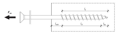
Figure 5.5: Screw insertion in timber specimen – definition of length parameters
