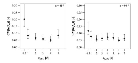
Figure B.48:CIs of  $CV[ln(f_{ax})]$  in dependence of spacing type and axis-to-grain angle; test specimen<br/>corresponding to section 5-4.1, test data from Gatternig (2010); (continued)
