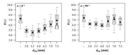
*Figure 5.86:* Boxplot diagrams of ductility D vs.  $d_{PD}$ ; left:  $\alpha = 0^\circ$ ; right:  $\alpha = 90^\circ$ ; test data from Gasser (2017)
