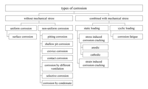
*Figure 3.69:* Classification of corrosion types; basing on Nürnberger (1995), Roos and Maile (2011) and Gläser et al. (2013)
