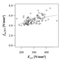
*Figure 5.25:* Comparison of selected withdrawal and clear wood properties for tangential screw axis orientation (continued)
