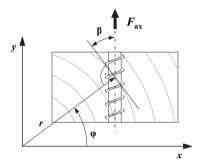
Figure 5.105: Definition of screw axis position with respect to annual ring orientation
