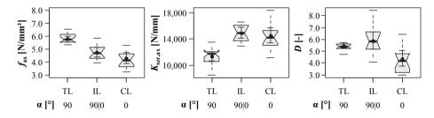
*Figure 5.99:* Boxplot diagrams of screw withdrawal properties when situated in intermediate layers; test data from Grabner (2013); d = 8 mm,  $\alpha = 90|0^{\circ}$
