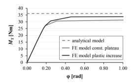
Figure 3.46: Numerically determined moment-rotation curves for the screw thread loaded in torsion
