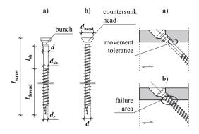
*Figure 2.33:* Comparison: (a) modified with (b) standard screw geometry; according to Ringhofer et al. (2014b)
