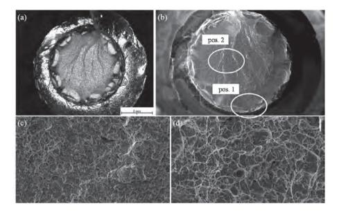
*Figure 3.63:* SEM images of a screw failed at N = 4,340; (a) photo of the fracture pattern; (b) microscopic scan with zoom positions; (c) zoom view of pos. 1; (d) zoom view of pos. 2; 500x magnification
