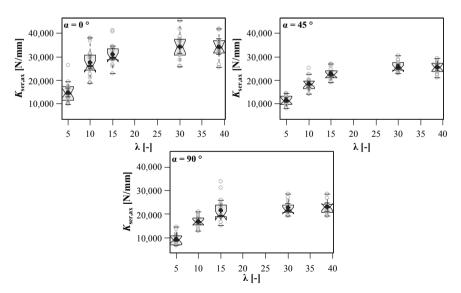
*Figure 5.113:* Combined boxplot/scatterplot graphics of withdrawal stiffness  $K_{ser,ax}$  in dependence of slenderness and axis-to-grain angle
