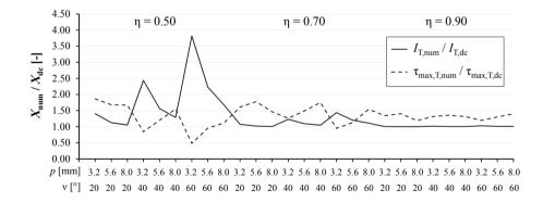
*Figure 3.21:* Ratios between cross-sectional screw thread torsional moments of inertia and maximum shear stresses due to uniform torsion and those of the inner thread's cylinder for varying parameters  $\eta$ , p and v, d = 8 mm
