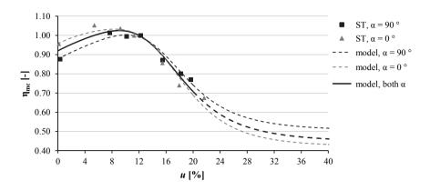
Figure 5.35: Comparison of the nonlinear model approach with test results of experimental campaign I
