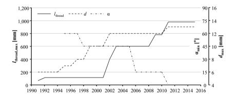
Figure 2.22: Development of thread length, outer thread diameter and minimum insertion angle between 1990 and 2014; only NTAs considered
