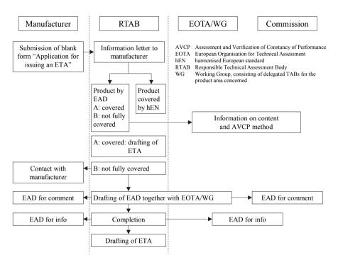
Figure 2.13: Procedure for drafting a European Assessment Document, according to DIBt (2015c)
