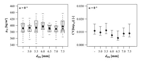
**Figure 5.79:** Left: boxplot diagram of densities  $\rho_{12}$ ; right: CIs of  $CV[ln(\rho_{12})]$  in dependence of  $d_{PD}$  for  $\alpha = 0$ °; test data from Gasser (2017)
