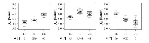
*Figure 5.100:* Boxplot diagrams of screw withdrawal strength  $f_{ax}$  when situated in intermediate layers; test data from Grabner (2013); d = 12 mm
