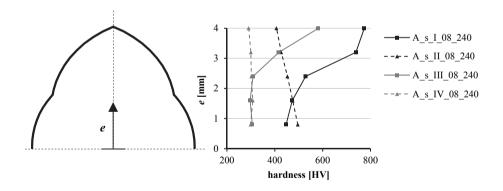
*Figure 3.44:* Varying hardness distributions over the screw thread profile determined by Toblier (2014) for product IDs A\_s\_I-IV\_08\_240
