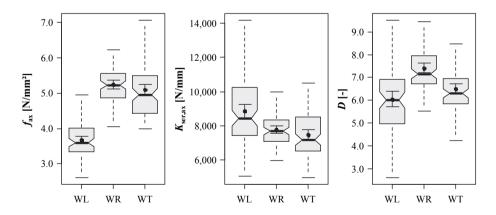
*Figure 5.16:* Boxplot diagrams of withdrawal strength (left), stiffness (middle) and ductility (right) vs. screw axis orientation
