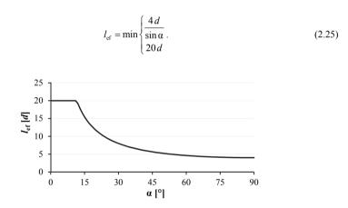
*Figure 2.14:* Effective inserted thread length (including the tip) as function of α; according to EAD 130118-00-0603 (2016)
