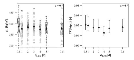
**Figure 5.66:** Left: combined boxplot/scatterplot graphic of densities  $\rho_{12}$ ; right: CIs of  $CV[ln(\rho_{12})]$  in dependence of spacing  $a_{2,CG}$  for axis-to-grain angle  $\alpha = 0^\circ$ ; test data from Gatternig (2010)
