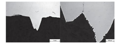
*Figure 3.81:* Micrograph of the advanced corrosion process, sample A\_s\_1\_08\_240 (yellow chromated) in oak as part of test campaign I; according to Hauptmann (2016)
