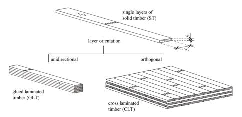
Figure 4.6: Definition of board-based layered timber products GLT and CLT
