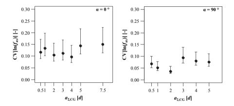
**Figure B.47:** CIs of  $CV[ln(f_{ax})]$  in dependence of spacing type and axis-to-grain angle; test specimen corresponding to section 5-4.1, test data from Gatternig (2010)
