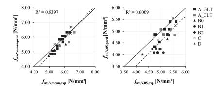
Figure 5.49: Experimental vs. predicted withdrawal strengths; left: mean values; right: 5 %-quantiles
