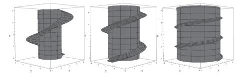
*Figure 3.19:* 3D illustration of thread geometries for three selected screw thread parameter sets, d = 8 mm; left: p = 8.0 mm,  $v = 20^\circ$ ,  $\eta = 0.50$ ; middle: p = 5.6 mm,  $v = 40^\circ$ ,  $\eta = 0.70$ ; right: p = 3.2 mm,  $v = 60^\circ$ ,  $\eta = 0.90$
