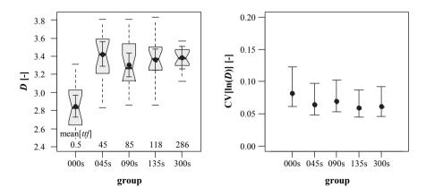
*Figure 5.126:* Left: boxplot graphic of ductility D; right: CIs of CV[ln(D)], both in dependence of time-to-failure (ttf)
