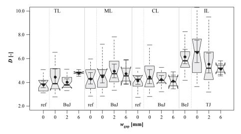
*Figure 5.58:* Boxplot diagrams of ductility vs.  $w_{gap}$  in dependence of screw position and gap type; test programme I, d = 8 mm
