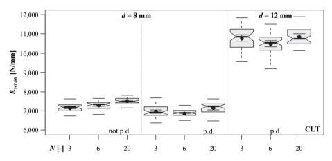
*Figure 5.45:* Boxplot diagrams of withdrawal stiffness vs. N in dependence of d and pre-drilling; test series A, CLT
