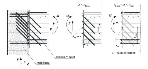
*Figure 2.37:* Left: cross-section of the aluminium-to-timber system connector "SHERPA"; middle and right: secondary beam force systems for an eccentric load introduction in dependence of e<sub>limit</sub>; according to Augustin (2011)
