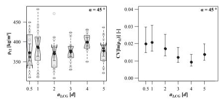
**Figure 5.67:** Left: combined boxplot/scatterplot graphic of densities  $\rho_{12}$ ; right: CIs of  $CV[[n(\rho_{12})]$  in dependence of spacing  $a_{2,CG}$  for axis-to-grain angle  $\alpha = 45^\circ$ ; test data from Gatternig (2010)
