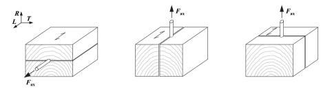
*Figure 5.1:* Schematic illustration of cut views made for the observation of withdrawal failure; left: LT-plane; middle: RL-plane; right: RT-plane
