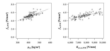
Figure 5.19: Comparison of selected withdrawal and clear wood properties for radial screw axis orientation
