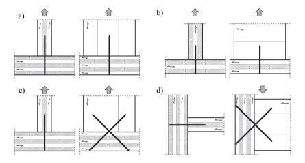
*Figure 6.8:* Overview of screwed CLT connections tested by Bratulic et al. (2014a): (a) and (b) exclusively axially loaded self-tapping screws; (c) and (d) predominately axially loaded self-tapping screws; according to Ringhofer et al. (2015a)
