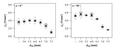
**Figure 5.82:** Boxplot diagrams of withdrawal strength  $f_{ax}$  vs.  $d_{PD}$ ; left:  $\alpha = 0$ °; right:  $\alpha = 90$ °; test data from Gasser (2017)
