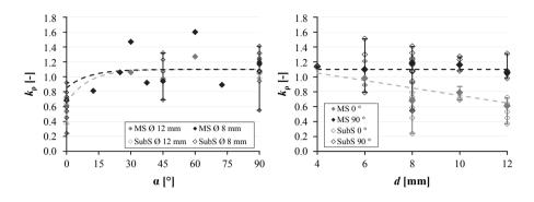
Figure 6.1:Exponent  $k_{\rho}$  vs. axis-to-grain angle  $\alpha$  (left) and outer thread diameter d (right); MS = main series;SubS = single subseries; Mod = model; according to Ringhofer et al. (2015c)
