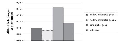
*Figure 3.91:* Diffusible hydrogen contents of three samples A\_s\_1\_08\_240, applied in oak, test campaign I (only steel)
