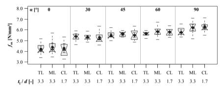
*Figure 5.94:* Boxplot diagram of withdrawal strength  $f_{ax}$  in dependence of axis-to-grain angle and ratio  $t_l / d$ ; test data from Grabner (2013); d = 12 mm
