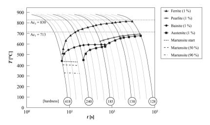
Figure 3.9: Example of a TTD for steel type 17B2; determined with JMatPro (2016)
