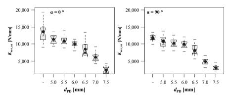
*Figure 5.84:* Boxplot diagrams of withdrawal stiffness  $K_{ser,ax}$  vs.  $d_{PD}$ ; left:  $\alpha = 0$  °; right:  $\alpha = 90$  °; test data from Gasser (2017)
