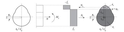
*Figure 3.28:* Stress distribution in the axially loaded screw's threaded part's cross-section with assumed ideal plastic material behaviour
