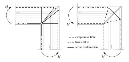
*Figure 2.38:* Assumed strut-and-tie models for moment rigid frame corners with axially loaded self-tapping screws; left: positive moment; right: negative moment; according to Trautz and Koj (2009)
