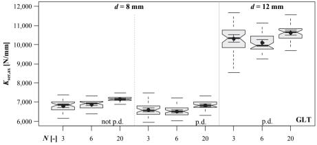
*Figure 5.44:* Boxplot diagrams of withdrawal stiffness vs. N in dependence of d and pre-drilling; test series A, GLT
