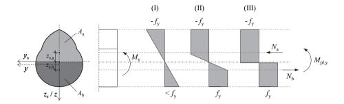
*Figure 3.24:* Different states of normal stresses due to pure bending (M<sub>y</sub>) at the screw's threaded part's crosssection: (I) yield strength reached at outer fibre; (II) intermediate state of cross-section plasticisation; (III) theoretical limit state of full plasticity
