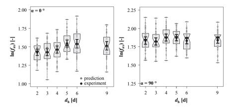
Figure 5.120: Logarithmic withdrawal strength in dependence of axis-to-grain angle and the supporting plate's hole diameter; according to Ringhofer and Schickhofer (2014a)
