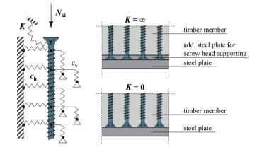
Figure 2.43: Left: assumed model for determining corresponding buckling loads; right: different forms of screw insertion as reinforcement of beam supports: screw head clamped in an additional steel plate (above); screw head placed in the timber member (below); according to Bejtka (2005)
