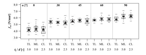
*Figure 5.93:* Boxplot diagram of withdrawal strength  $f_{ax}$  in dependence of axis-to-grain angle and ratio  $t_l / d$ ; test data from Grabner (2013); d = 8 mm
