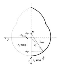
*Figure 3.33:* Relationship between r<sub>shear</sub> and r<sub>c</sub> for the given screw thread profile
