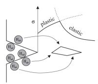
Figure 3.71: Crack formation close to surface discontinuities due to HISCC, according to Gräfen and Kuron (1987)
