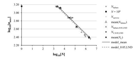
*Figure 3.59:* Bearable load cycles in dependence of N in case of R = 0.56
