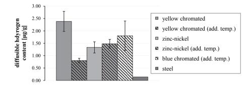
Figure 3.54: Diffusible hydrogen contents determined for varying protective coats
