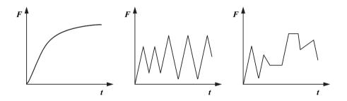
*Figure 3.55:* Different load-time-relationships in the pulsating tensile domain: left: monotonic loading; middle: cyclic loading; right: random loading
