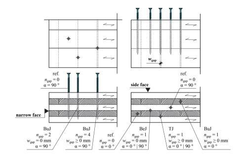
*Figure 5.50:* Screw insertion in CLT components with respect to specific product characteristics; left: side face insertion; right: narrow face insertion
