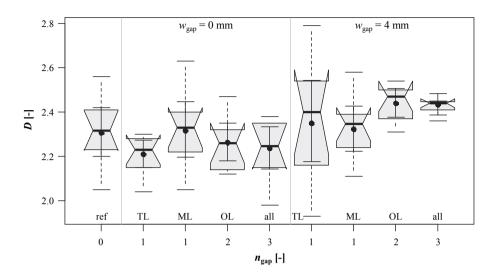
Figure 5.62: Boxplot diagrams of ductility vs. w<sub>gap</sub> and n<sub>gap</sub>; test programme II
