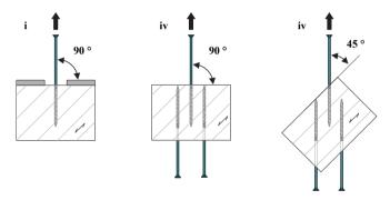
Figure 5.118: Schematic overview of campaign III parameter variation; according to Ringhofer and Schickhofer (2014a)
