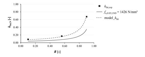
Figure 3.60: Comparison of experimentally determined values for  $k_{fat}$  with the model assumption and "detail category 50" according to ON EN 1993-1-9 (2013)
