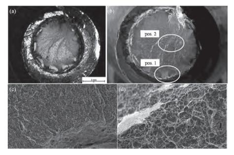
*Figure 3.62:* SEM images of a screw failed at N = 1,766; (a) photo of the fracture pattern; (b) microscopic scan with zoom positions; (c) zoom view of pos. 1; (d) zoom view of pos. 2; 500x magnification
