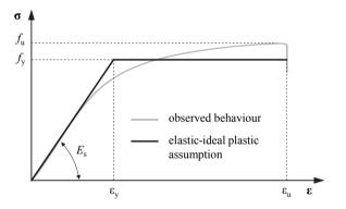
Figure 3.23: Observed and assumed stress-strain-relationship of a carbon steel screw loaded in tension
