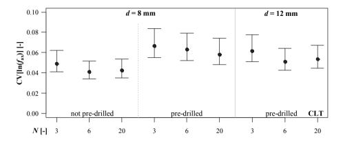
**Figure B.28:** CIs of  $CV[ln(f_{ax})]$  in dependence of N, d and pre-drilling; series A, CLT; test specimen corresponding to section 5-3.3
