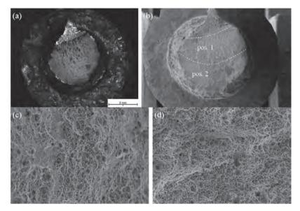
*Figure 3.85:* A\_s\_IV\_08\_240 (zn) in oak; (a) fracture pattern; (b) SEM scan with zoom positions; (c) zoom view of pos. 1; (d) zoom view of pos. 2; 500x magnification; according to Hauptmann (2016)
