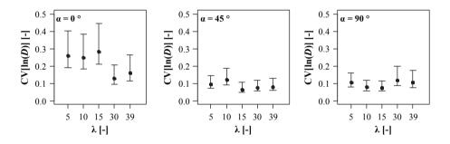
*Figure B.71:* CIs of CV[ln(D)] in dependence of axis-to-grain angle and slenderness; test specimen corresponding to section 5-4.5
