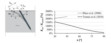
**Figure 2.30:** Left: lateral and axial displacement components of inclined screw joints; according to Tomasi et al. (2010); right: comparison of connection stiffness  $K_{ser}$  (referred to  $K_{ser,lad}$ ) between the models of Blaß et al. (2006) and Tomasi et al. (2010)
