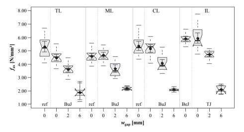
*Figure 5.56:* Boxplot diagrams of withdrawal strength vs.  $w_{gap}$  in dependence of screw position and gap type; test programme I, d = 8 mm
