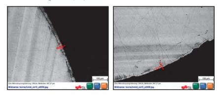
Figure 3.12: Micrographs of two cut screw thread cross-sections for determination of coating thickness
