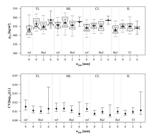
*Figure 5.53:* Above: boxplot graphic of densities  $\rho_{12}$ ; below: CIs of  $CV[ln(\rho_{12})]$  in dependence of gap type and width; test programme I, d = 8 mm
