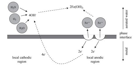
Figure 3.67: Schematic illustration of metal (steel) corrosion in aerated water (primary reaction); basing on Nürnberger (1995)
