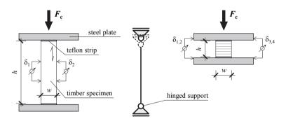
*Figure 5.14:* Clear wood compression tests according to ON EN 408 (2010); left and right: schematic illustration of the test set-ups with load application in longitudinal and radial direction; middle: corresponding static system
