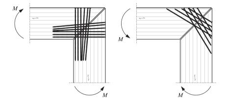
Figure 2.39: Arrangement of self-tapping screws responsible for tensile load transmission; left: positive moment; right: negative moment; according to Trautz and Koj (2009)
