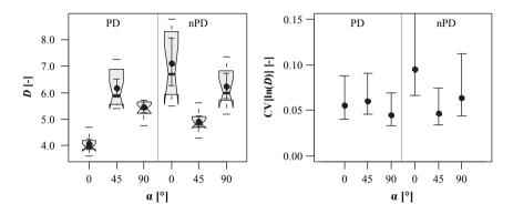
*Figure 5.85:* Left: boxplot diagram of ductility D; right: CIs of CV[ln(D)]; both in dependence of axis-to-grain angle and pre-drilling, test data from Grabner (2013)
