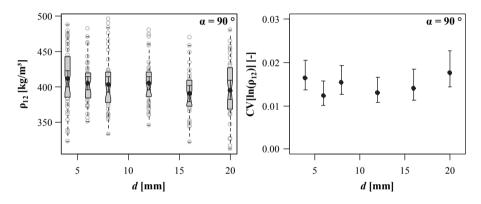
*Figure 5.10:* Left: combined boxplot/scatterplot graphic of densities  $\rho_{12}$ ; right: Cls of  $CV[[n(\rho_{12})]; \alpha = 90^{\circ}$
