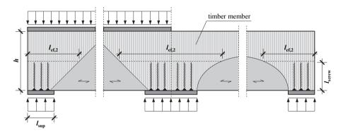
Figure 2.42: Different loading and supporting situations for beam supports reinforced with self-tapping screws: left: directly loaded end support; middle: support with both load situations; right: indirectly loaded end support; according to Bejtka and Blaß (2006)
