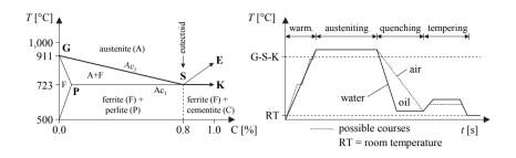
*Figure 3.8:* Left: extract of the iron-carbon diagram, including the G-S-K line; right: four phases of hardening in the temperature-time diagram; according to Weiβbach (2012)
