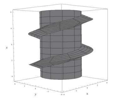
Figure 3.14: 3D illustration of an exemplarily determined screw thread profile
