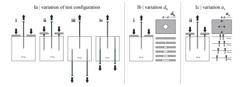
*Figure 5.117:* Schematic overview of campaign I parameter variation exemplarily for  $\alpha = 90^\circ$ ; according to Ringhofer and Schickhofer (2014a); (i) push-pull, (ii) push-pile, (iii) pull-pull, (iv) pull-pile
