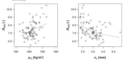
Figure 5.22: Comparison of selected withdrawal and clear wood properties for radial screw axis orientation (continued)
