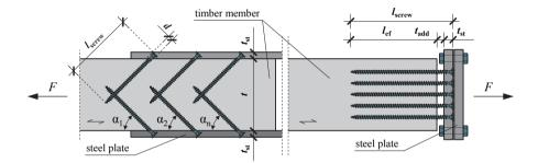
Figure 2.32: Cross-section of two types of steel-to-timber connections with predominately axially loaded selftapping screws; left: inclined screw butt joint; right: end-grain joint with screws inserted parallel to grain direction
