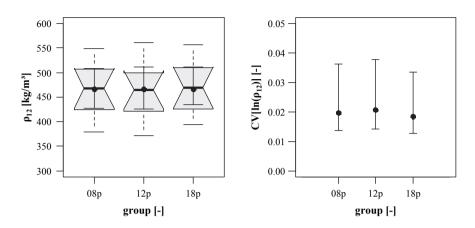
*Figure 5.29:* Left: boxplot graphic of densities  $\rho_{12}$ ; right: CIs of  $CV[ln(\rho_{12})]$  in dependence of moisture content groups;  $\alpha = 90^\circ$ , experimental campaign II
