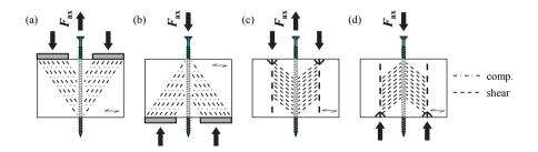
*Figure 5.116:* Examples of different loading and supporting conditions for screw withdrawal tests according to Gehri and Haas (2008); (a) and (c) loaded in tension, (b) and (d) loaded in compression
