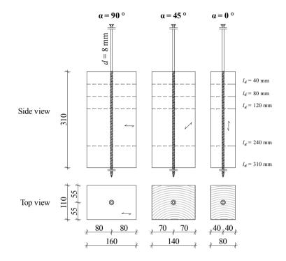
Figure B.68: Illustration of test specimen corresponding to section 5-4.5; all dimensions in [mm]
