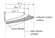
Figure 5.87: Schematic illustration of the reduced contact surface due to pre-drilling
