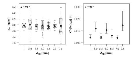
**Figure 5.80:** Left: boxplot diagram of densities  $\rho_{12}$ ; right: CIs of  $CV[ln(\rho_{12})]$  in dependence of  $d_{PD}$  for  $\alpha = 90^{\circ}$ ; test data from Gasser (2017)
