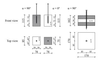
*Figure B.19:* Illustration of withdrawal test specimen corresponding to section 5-3.2; left: experimental campaign I; right: experimental campaign II; according to Ringhofer et al. (2014c); all dimensions in [mm]
