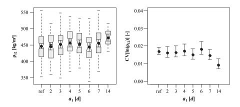
*Figure 5.70:* Left: boxplot diagram of densities  $\rho_{12}$ ; right: CIs of  $CV[ln(\rho_{12})]$  in dependence of spacing  $a_1$ ; test data from Plieschounig (2010);
