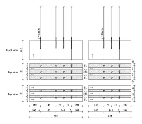
Figure B.34: Illustration of test specimen corresponding to section 5-3.4, test campaign I; exemplarily for d = 8 mm; all dimensions in [mm]
