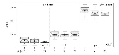
Figure 5.46: Boxplot diagrams of ductility vs. N in dependence of d and pre-drilling; test series A, GLT
