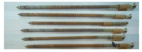
Figure B.11: Macrophotos of A\_s\_II\_08\_240 (yellow chromated) applied in oak; test campaign II
