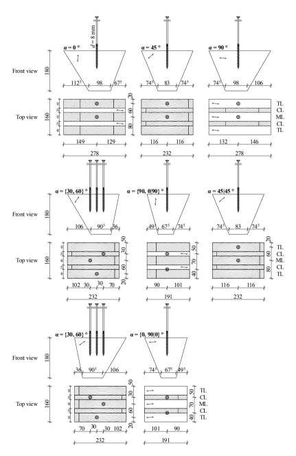
*Figure B.59:* Illustration of test specimen corresponding to section 5-4.3, test campaign I; exemplarily for d = 8 mm; all dimensions in [mm]
