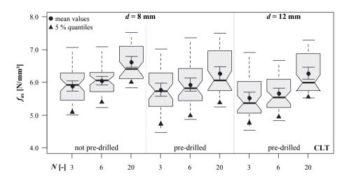
*Figure 5.43:* Boxplot diagrams of withdrawal strength vs. N in dependence of d and pre-drilling; test series A, CLT
