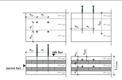
Figure 2.12: Minimum distances of predominately axially loaded screws in CLT side and narrow faces; according to ON B 1995-1-1 (2014)
