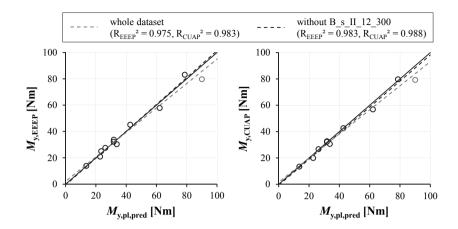
*Figure 3.47:* Comparison of experimentally determined and predicted values for M<sub>y</sub>; left: M<sub>y</sub> determined according to ASTM E2126 (2002); right: M<sub>y</sub> determined according to Blaβ et al. (2000) and CUAP 06.03/08 (2010)
