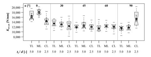
*Figure 5.95:* Boxplot diagram of withdrawal stiffness  $K_{ser,ax}$  in dependence of axis-to-grain angle and ratio  $t_1/d$ ;test data from Grabner (2013); d = 8 mm
