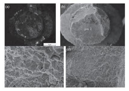
*Figure 3.87: A\_s\_1\_08\_240 (yc) in oak; (a) fracture pattern; (b) SEM scan with zoom positions; (c) zoom view of pos. 1 (1000x); (d) zoom view of pos. 2 (500x magnification); according to Hauptmann (2016)*
