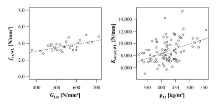
*Figure 5.18:* Comparison of selected withdrawal and clear wood properties for longitudinal screw axis orientation (continued)
