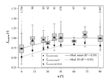
**Figure 6.2:** Behaviour of density-corrected and normalised withdrawal strength  $f_{ax,norm}$  in dependence of axis-to-grain angle a; according to Ringhofer et al. (2015c)
