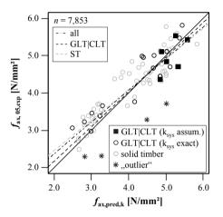
*Figure 6.9:* Comparison of empirical 5 %-quantiles of all test series with characteristic (5 %) withdrawal strengths determined by eq. (6.20); according to Ringhofer et al. (2015a)
