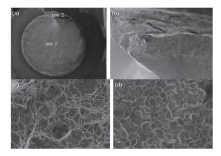
*Figure 3.86: A\_s\_I\_08\_240 (yc) reference; (a) SEM scan with zoom positions; (c) zoom view of pos. 1; (1000x) (b) and (d) zoom view of pos. 2; (100x/1000x magnification); according to Hauptmann (2016)*
