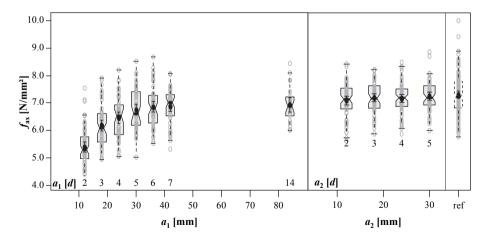
*Figure 5.73:* Combined boxplot/scatterplot diagram of withdrawal strength vs. spacing  $a_1$  and  $a_2$ ; test data from Plieschounig (2010)
