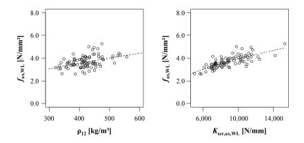
Figure 5.17: Comparison of selected withdrawal and clear wood properties for longitudinal screw axis orientation
