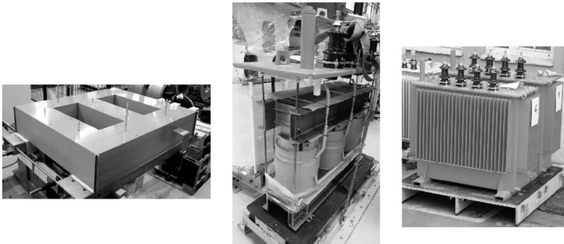
Figure 11.15: Model transformer core, active part, and uniform tank.
