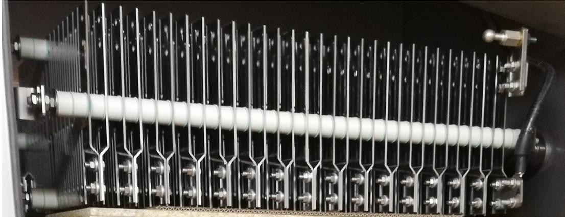
Figure 26: Detail view of LONE resistor
