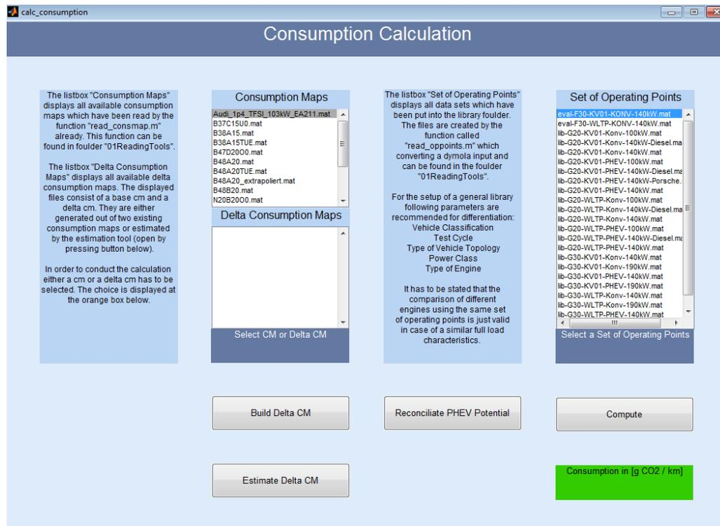
Figure 3.23: Central control panel of Ventus-Tool.
