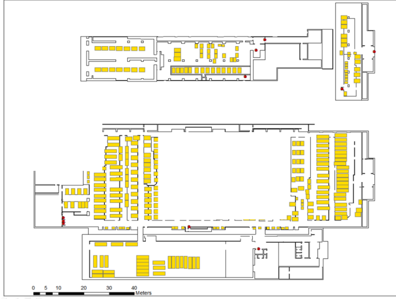
Figure 1. Indoor space layout of the semiconductor production subject of this paper. Equipment is represented by yellow rectangles and transfer points are denoted with red dots. White spaces are included intentionally to disguise the production layout.
