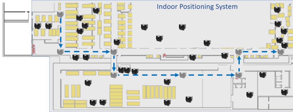
Figure 1.1: Topological model of the indoor production environment including layout, equipment (yellow), production asset (boxes), movement (arcs) and the indoor positioning system.
