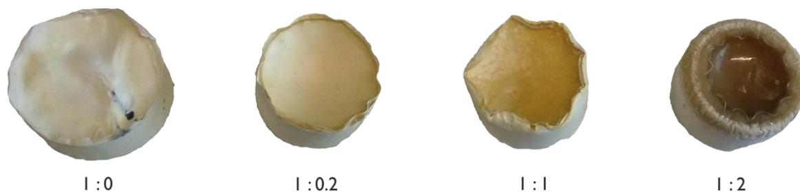
Figure 25: pDCPD monoliths synthesised with the HIPE procedure using different DCPD:cyclohexane ratios for the continuous phase. Samples are depicted after the drying step.
