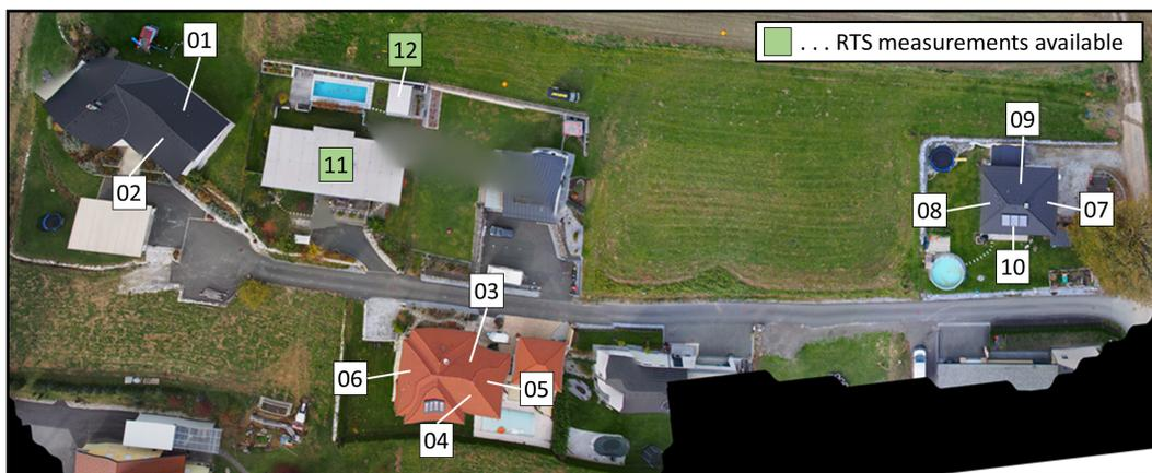
**Figure 4–12:** Rooftops used for investigation of orientation accuracy. For rooftops 11 and 12, not only photogrammetric measurements from both approaches, but also RTS measurements are available.
