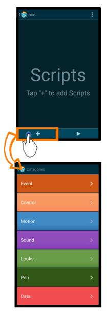
Figure 3.7.: Pocket Code's UI: add new scripts and choose bricks from the seven basic available categories.
