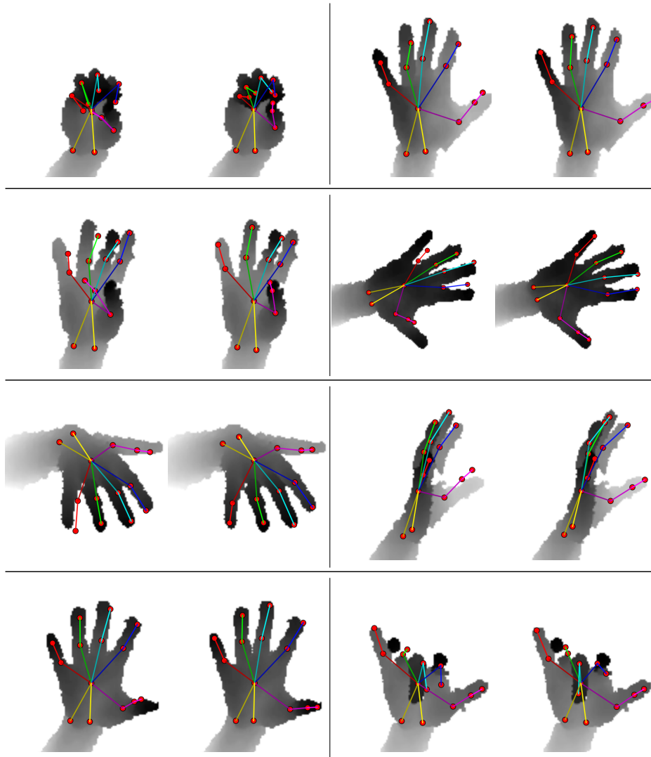
Figure 5.20: Qualitative results on NYU dataset [271]. We show the inferred joint locations on the depth images where the depth is color coded in gray-scale. The individual fingers are color coded, where the bones of each finger share the same color, but with a different hue. The left image of each pair shows the initialization and the right image shows the pose after applying our feedback method. Our method applies to a wide variety of poses and is tolerant to noise, self-occlusions and missing depth values as shown in several images.
