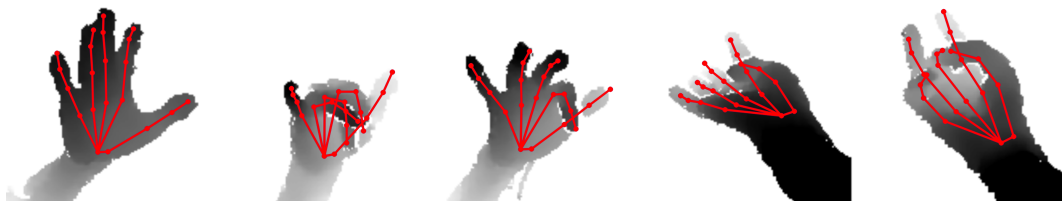
Figure 4.14: Qualitative results on the BigHands dataset [311]. We show the inferred 3D joint locations projected on the depth images. Since there is no publicly available ground truth for the test images available, we only show the predicted poses in red.
