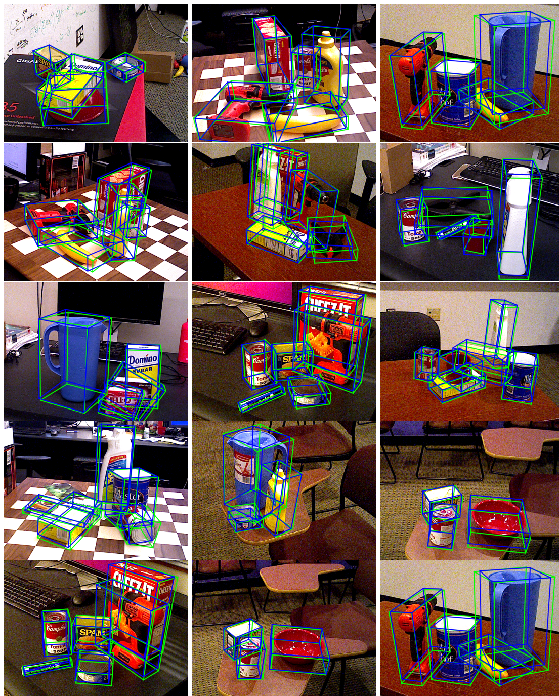
Figure 10.13: Qualitative results on the YCB-Video dataset [297]. The green bounding boxes correspond to the ground truth poses, the blue ones to our estimated poses.
