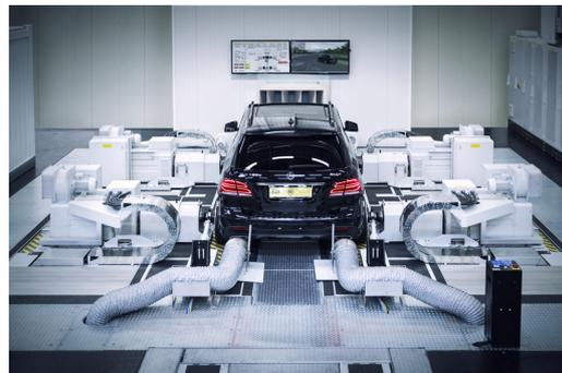
(b) KS R2R full vehicle Road to Rig test bed, © KS Engineers.
