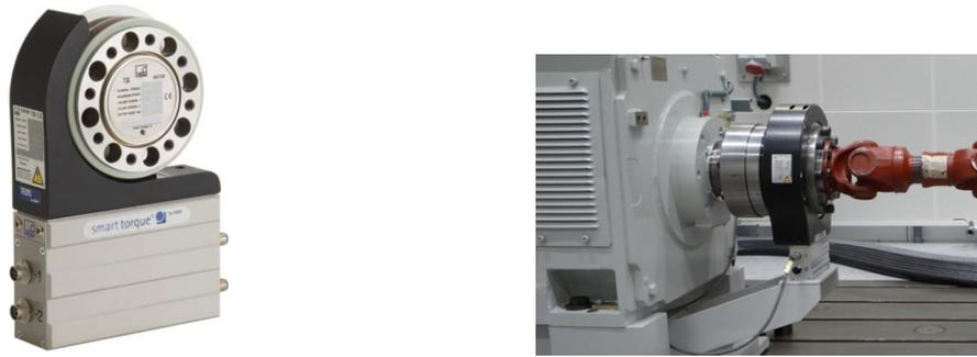
(a) Torque measuring flange HBM T12 [24]. (b) Torque sensor with covering attached to electric drive.
