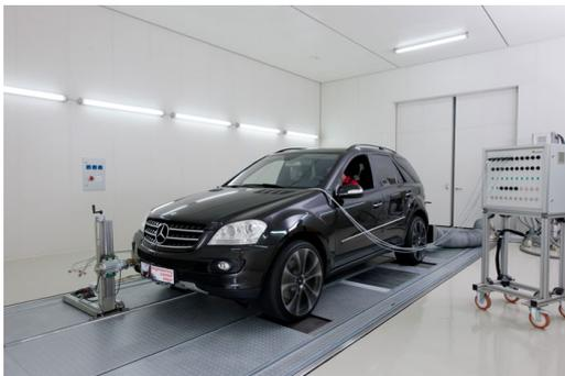
(a) Roller chassis dynamometer, © KS Engineers.
