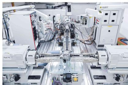
**Figure 2.3:** KS R2R power train test bed with electric input drive, © KS Engineers.
