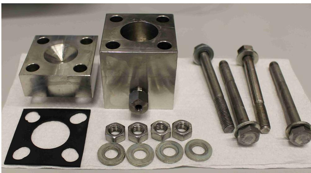
Figure 6.27: All parts of the reactor
