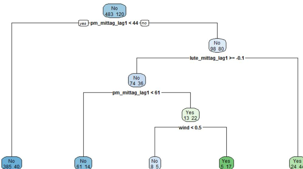
Figure 3.3: Pruned Binary Tree for Graz Mitte with  $\alpha = 0.02$
