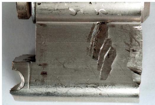
Fig. 1: Snapped lock with multiple toolmarks.
