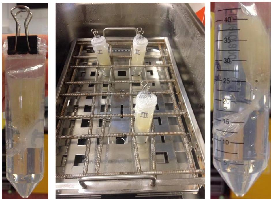
Figure 9 Centrifuge tubes with dialysis tubes, containing BG sample and bovine bile, fixed with binder clip (left, right). Dialysis experiment in shaking water bath (middle).
