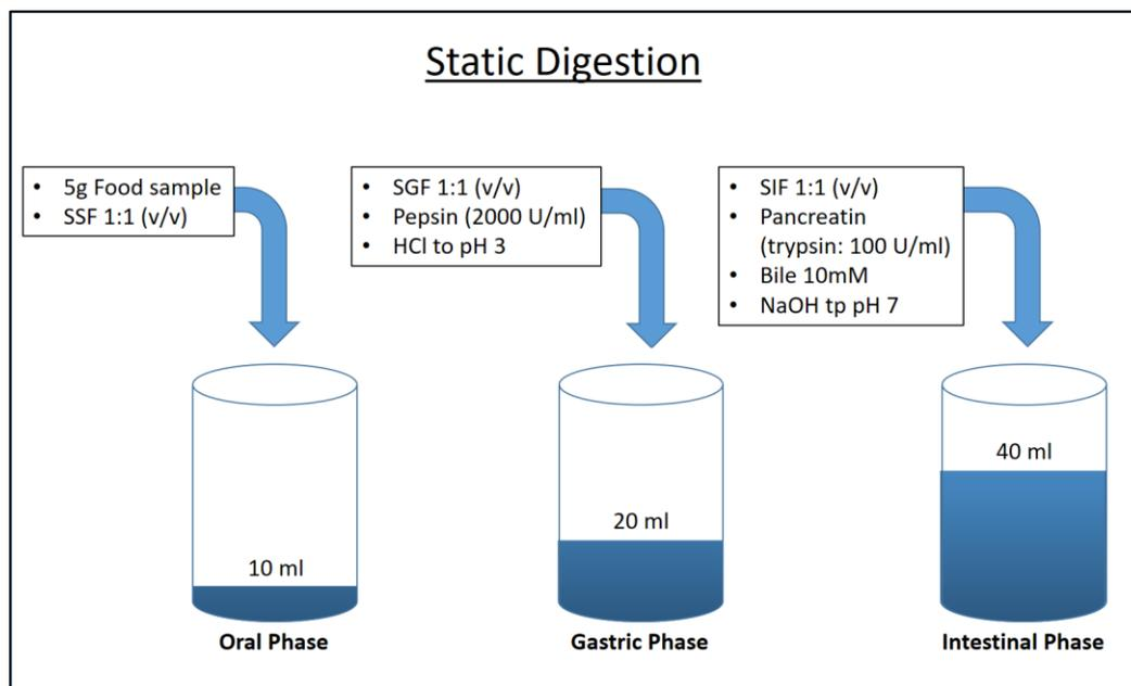
Figure 10 Schematic set-up of static digestion experiments.
