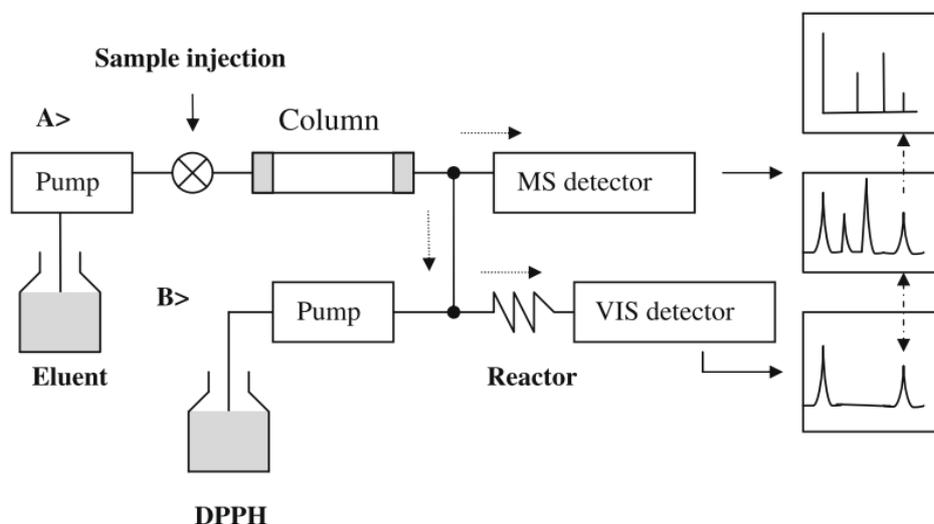
**Figure 3: On-line coupled HPLC-MS-DPPH assay [25]**
